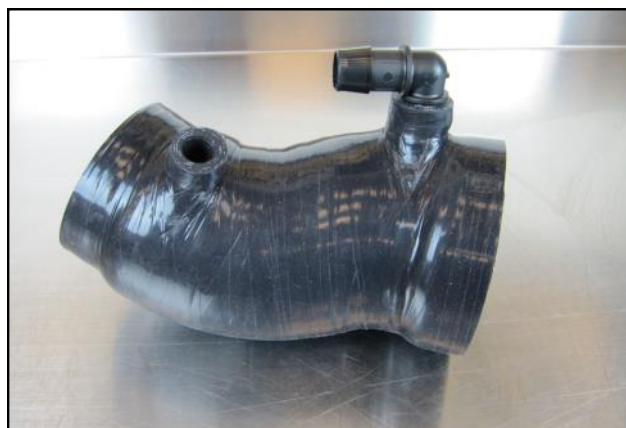
7. Insert the Barbed Elbow Connector into the Airaid Intake Tube as shown.
