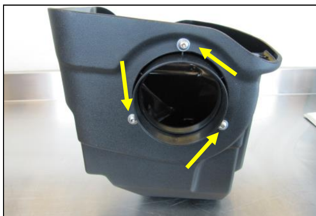
4. Install the Filter Adapter onto the Cool Air Box using the three 1/4" Button Head Screws and 1/4" Flat Washers.
