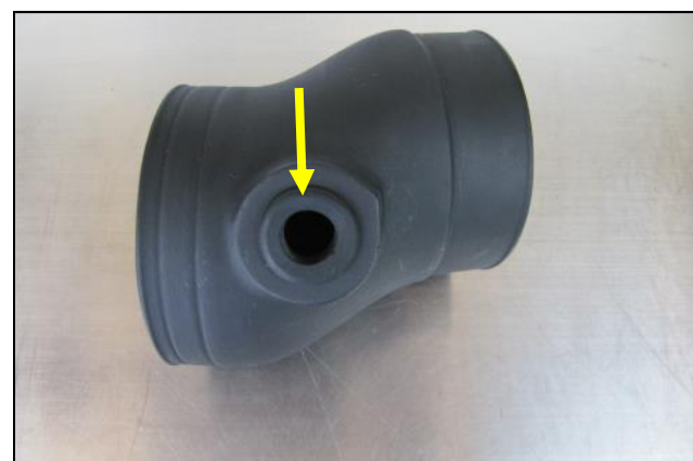
6. Insert the Grommet into the Intake tube.
