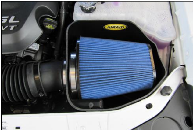
14. Install the Airaid Premium Filter onto the Filter Adapter.
