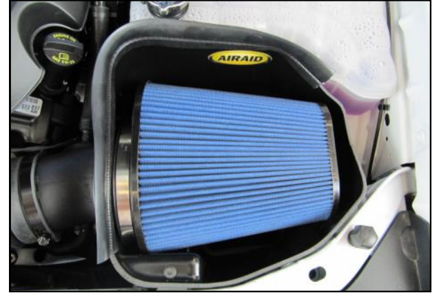
15. Install the Weatherstrip onto the top edge of the Air Box with the contour rolling away from the Filter.
