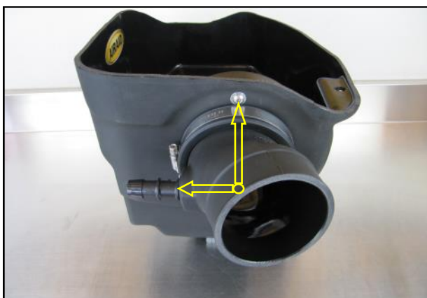
8. Install the Intake Tube into the Coupler as shown, with the Barbed Fitting in the Nine O'clock position. Do not tighten the Clamp at this time.
