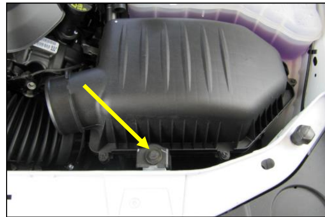
3. Remove the air box screw in the core support and lift the air box out of the vehicle. Set the screw aside, it will be reused in step 11.
