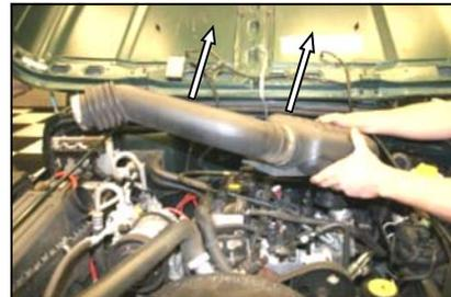
2. Remove the intake tube and resonator from the vehicle.
