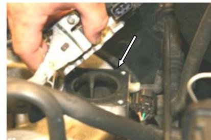
4. With the throttle body set aside, remove the gasket and clean the surfaces of the manifold and throttle body.
