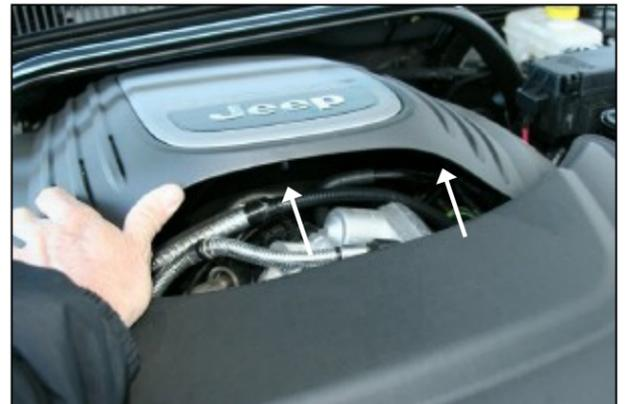
**6.** Carefully lift up on the engine cover (*it is held in place by grommets, no bolts*) to access the hose clamp on the throttle body, and 10mm bolt next to the throttle body.
