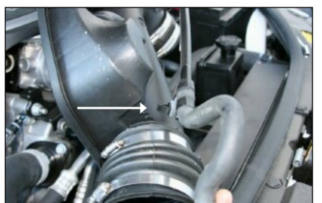
**9.** Slide the clip off of the resonator that holds the breather tube in place.
