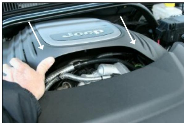
20. Realign the engine cover with the grommets on the engine, and push down firmly to reseal the cover.
