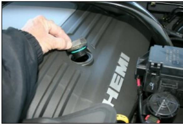
**5.** Remove, and set aside the oil filler cap. *Use caution not to drop anything into engine while cap is off.*
