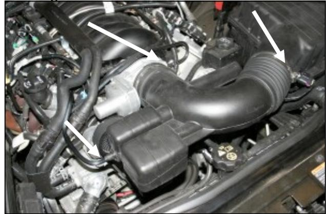
**2. Disconnect the breather hose elbow by pulling it straight away from the intake tube. It is only held in place by an O-ring. Loosen the two hose clamps that secure the intake tube to the throttlebody, and the air box lid. Remove the air intake tube.**
