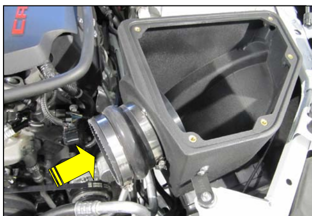
19. Slide the Hump Hose and #68 Clamps onto the Filter Adapter.
