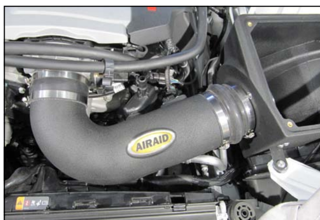
22. Align the Intake Tube and tighten all four Clamps.
