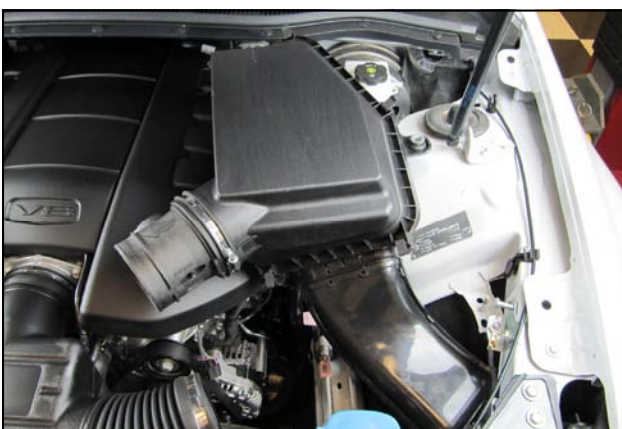
4. Separate the intake tube from the Mass Air Flow sensor and remove the entire air box assembly from the vehicle.
