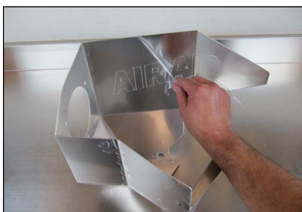
5. Carefully remove the protective film from both sides of the Air Dam.
