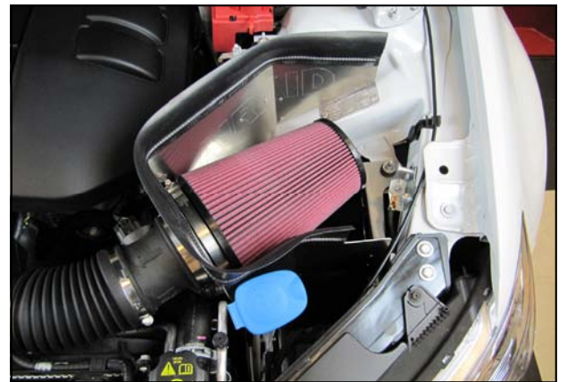
15. Install the Weatherstrip onto the top edge of the Air Dam with the contour rolling away from the Filter.
