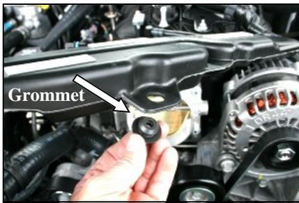
7. Remove the factory grommet from the intake tube.
