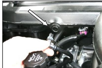
2. Disconnect the breather tube from the intake tube, by gently pulling towards you. An O-ring is all that holds it in place. Next loosen the hose clamp on the intake tube at the throttle body, and at the Mass Air Sensor, and remove the tube from the vehicle.
