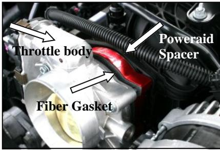
5. Install 2 of the supplied bolts (#2) and washers (#3) thru the two holes in the top of the throttle body, thru the supplied fiber gasket (#4), thru the Poweraid Spacer, and into the two brass inserts in the intake manifold. Run the bolts in a few threads with your fingers. Use caution not to cross-thread the bolts. Next install the 2 remaining bolts (#2) and washers (#3) in the two bottom holes of the throttle body, and tighten in a cross pattern to the vehicle manufacturer's specifications.
