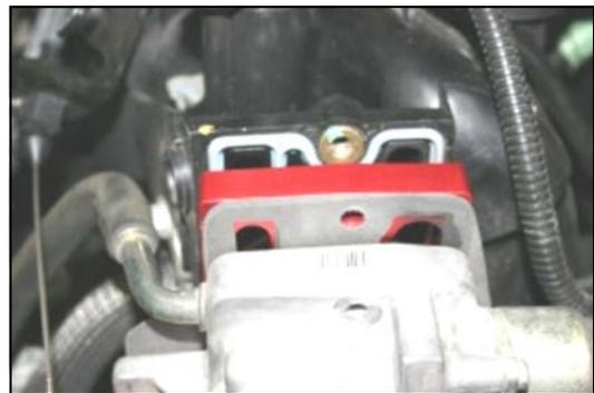
6. Make sure the direction of the airflow is correct on the Poweraid Spacer (#1), then with the gasket (#4) on the throttle body side, slide the Poweraid between the throttle body and the intake manifold. Install the top bolt (#2) and washer (#3) first, then the two bottom bolts and washers.
