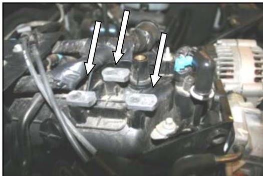
5. Install the three linkage plates (#5) with the three flat head screws (#6) as shown, pointing towards the front of the vehicle.
