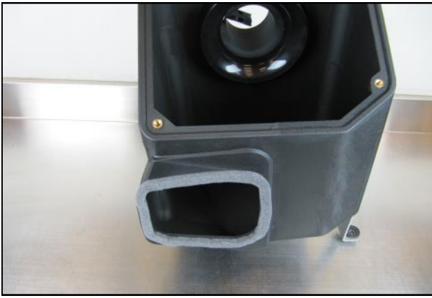
10. Prepare the Air Box for the weather Seal by cleaning the outer edge with a prep-sol or equivalent. Apply the self adhesive, Foam Weather Seal onto the Air box inlet as shown.
