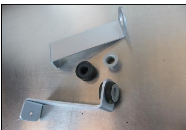
8. Transfer OEM air box bushings and anti-crush sleeves into the Airaid Air Box Brackets as shown.
