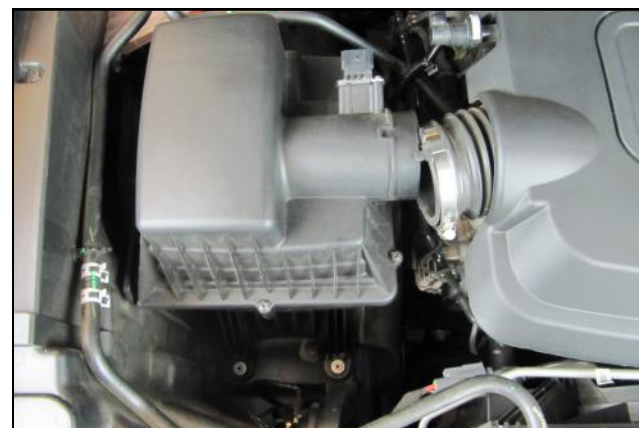
3. Loosen the intake clamp and slide the tube off of the air box lid as shown. Using a screwdriver, remove the air box lid and air filter.
