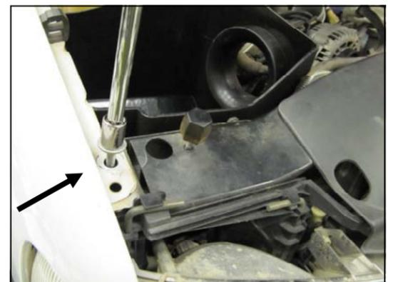
**6. Using a 13mm socket, remove the factory fender bolt** and set it aside. It will be reused in step 7.
