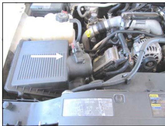
**2. Disconnect the Mass Air Flow (M.A.F.) sensor** and remove the factory airbox. Rock the factory air box back and forth and remove it from its mounting. It is held in place with grommets.
