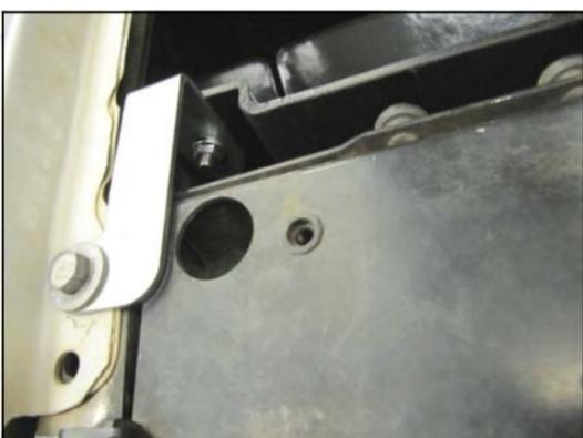
**7. Install the Fender bracket (#13) as shown. A.)** Secure the bracket to the fender using the factory bolt. **B.)** Use the 1/4-20 x 3/4" hex bolt (#14), one 1/4" flat washer (#9), and the 1/4-20 flange nut (#15) to secure the CAB to the Bracket.
