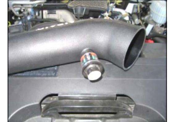
**9. Transfer the factory rubber grommet and air filter minder from the airbox top into the Airaid intake tube** As shown.
