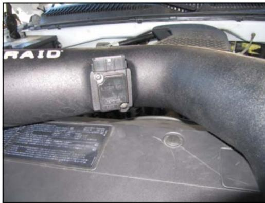
**8. Transfer the M.A.F. Sensor from the factory airbox into the Airaid intake tube (#2).** Use the two 8-32 button head screws (#10), to secure the meter. **Do Not Use Factory Screws.**
