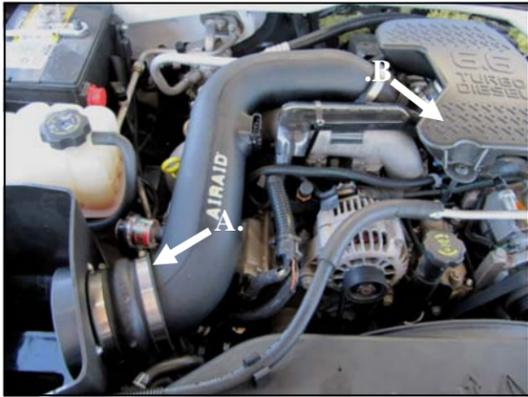
**14.** A.) Install the hump hose end of the Airaid intake tube assembly onto the filter adapter first. B.) Slip the coupler end of the tube over the factory turbocharger inlet. Adjust for fit, and tighten the hose clamps
