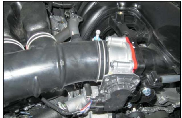
6. Reinstall the factory intake tube, tighten the two hose clamps, and reconnect the crankcase breather and Fuel pressure regulator lines. Reinstall the engine cover.
