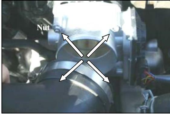
3. Using a 10mm socket, remove three factory bolts, and one nut. Pull the throttle body towards the radiator until it clears the stud, and then move it aside.
