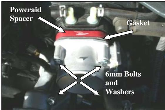
5. Position the Poweraid Spacer (#1) and gasket (#2) between the throttle body and intake manifold. Insert four 6mm x 65mm hex bolts (#3), and 6mm flat washers (#4) thru the throttle body, gasket, Poweraid Spacer, and into the intake manifold. Using a 10mm socket, tighten all four throttle body bolts evenly, to the manufacturers specifications. **Do Not Over Tighten The Bolts!**
