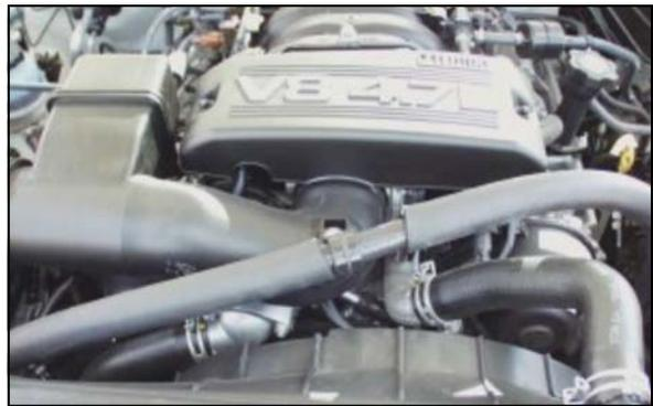
6. Re-install the intake tube and tighten the hose clamps. Re-connect the vacuum lines, wiring harness clip, and breather hose. Re-install the bolt thru the clamp on the air conditioning hose into the intake tube. Re-install the beauty cover and nuts.
