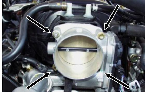
4. With a 10mm socket, remove three bolts and one nut from the throttle body. Slide the throttle body away from the intake manifold, and remove the remaining stud.
