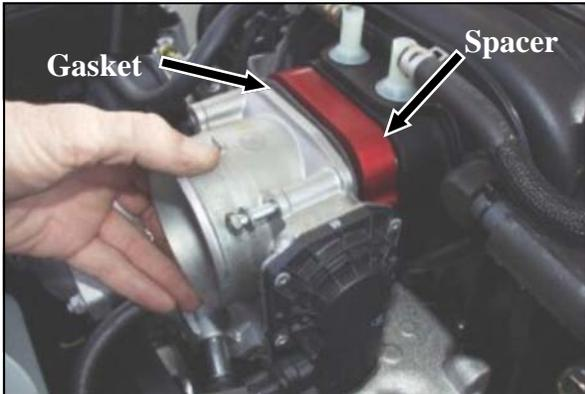
5. Install the Poweraid spacer (#1) next to the intake manifold, and the fiber gasket (#4) next to the throttle body. Insert the four provided 6mm bolts (#2), and washers (#3), and tighten in a cross pattern, to the vehicle manufacturer's specifications.
