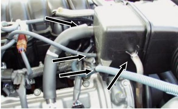
3. Disconnect the breather hose, and two vacuum lines from the back of the intake tube. Remove the clip from the back of the intake tube that holds the wiring harness, these will all be re-connected later. Remove the intake tube from the vehicle.
