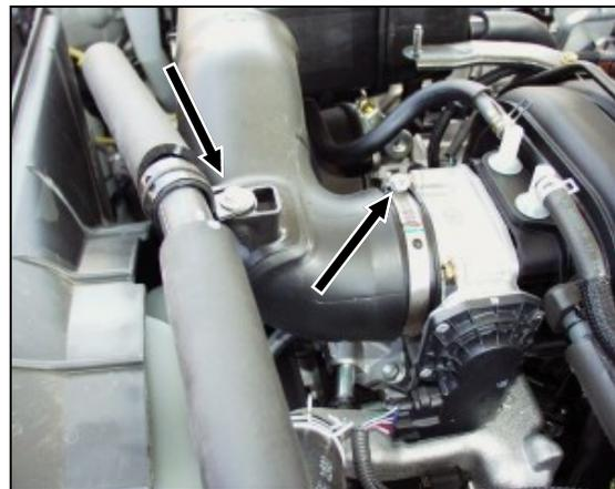
2. Loosen the hose clamp that holds the intake tube to the throttle body. Remove and save the bolt that holds the air conditioning line to the intake tube.
