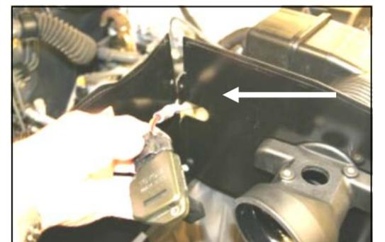
6. Remove the top screw on the CAD. Spread the panels slightly, and slip the wiring harness thru the gap into the access hole, as shown. Re-install the screw and tighten.
