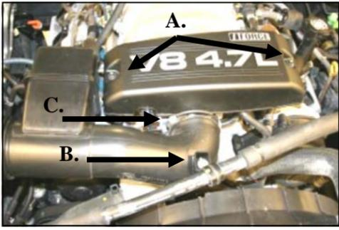
10. A) Using a 10mm socket, remove the two nuts and remove the beauty cover. (Save for reinstallation.) B) Remove the bolt thru the Adel clamp for the air conditioning hose. C) Loosen the hose clamp on the factory intake tube at the throttle body and the airbox if it was tightened in step #5.
