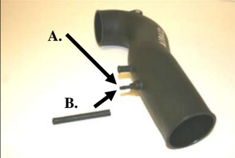
14. A) Install the 1/4" Barb x 1/8" NPT fitting (#14) into the Airaid Modular Intake Tube (MIT) (#5).
