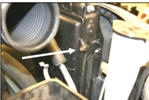
4. Remove the fan shroud bolt from the passenger side of the radiator. (Save for reuse).
