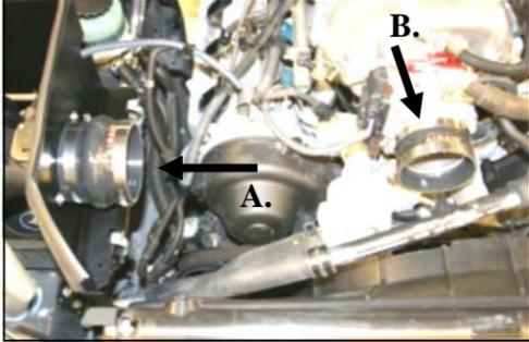
13. A) Install the urethane hump hose (#7) onto the MAF adapter (#4). Use the #56 hose clamp (#12) on the MAF adapter end, and the #60 hose clamp (#13) on the intake tube end. B) Install the reducer coupler (#6), small end towards the throttle body with two #52 hose clamps (#11). Leave the clamps loose for now.
