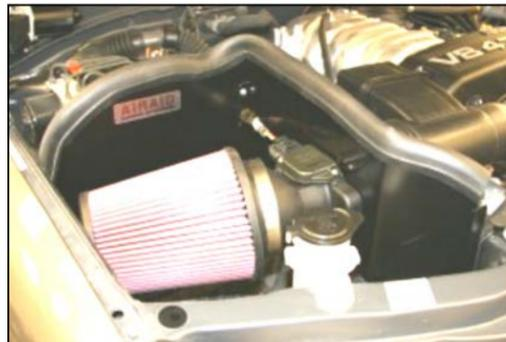
8. Install the Airaid Premium Filter (#1) onto the MAF adapter. Next install the weather strip (#10) on top of the CAD. Start at the radiator end and work your way towards the back.
