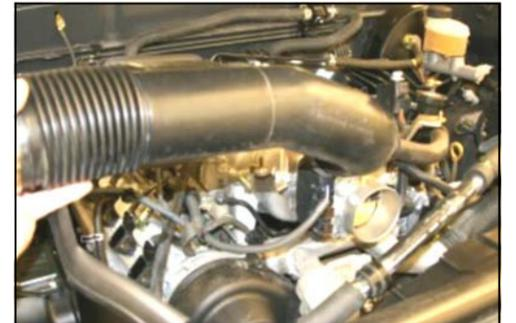
12. Remove the factory intake tube.
