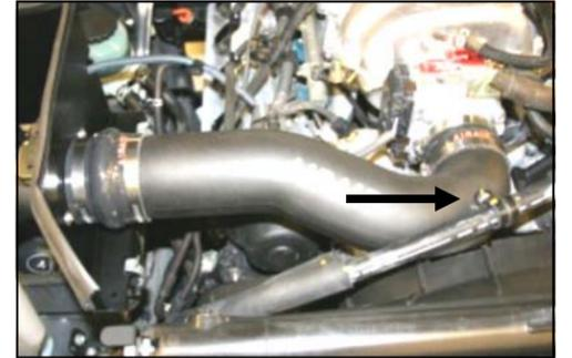
15. Install the Airaid MIT (#5) into the hump hose first, and then into the coupler. Adjust the MIT snugly against the throttle body and tighten all four clamps. Install the supplied button head bolt (#20), and washer (#21) thru the Adel clamp, and thread into the MIT. (See arrow)
