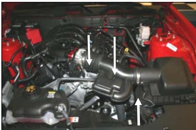
7. Reinstall the intake tube, tighten the two hose clamps, and reconnect the breather line or lines.
