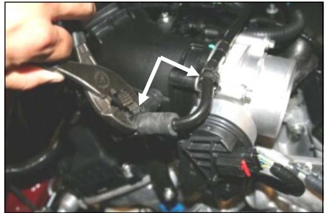
2. Using pliers, open the spring clamps and slide off of the factory breather hose, and onto the hard line.
