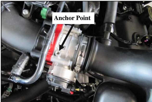
5. If your breather is a two piece line, disconnect the anchor from the throttle body to allow it to remain in position.
