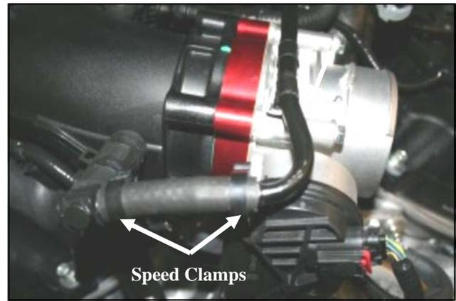
6. If you have a three piece breather hose and spring clamps, and replace them with the supplied Breather hose and Speed clamps. Re-torque the throttlebody bolts in a X pattern, to Factory specs.
