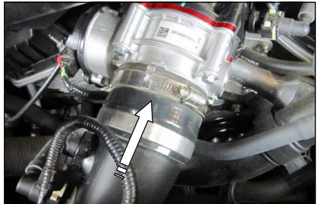
4. Slide the throttle body inlet tube back onto the throttle body and tighten the clamp.
