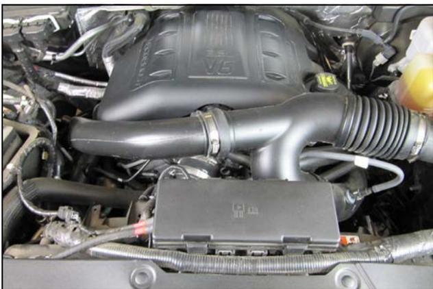
5. Reinstall the intake tube, and any other parts that were removed to gain access to the throttle body in the reverse order in which they were removed. Double check your work. Make sure there is no foreign material in the intake tract. Make sure all clamps, connectors, hoses, nuts, and bolts are secure.
