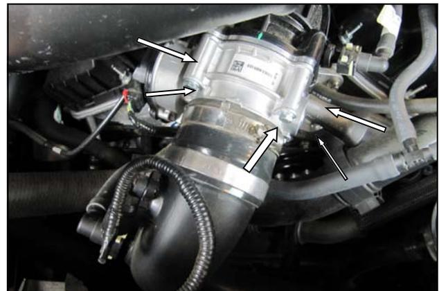
2. Loosen the clamp on the throttle body inlet tube and slide it away from the throttle body. Remove the four bolts that secure the throttle body to the intake manifold.
