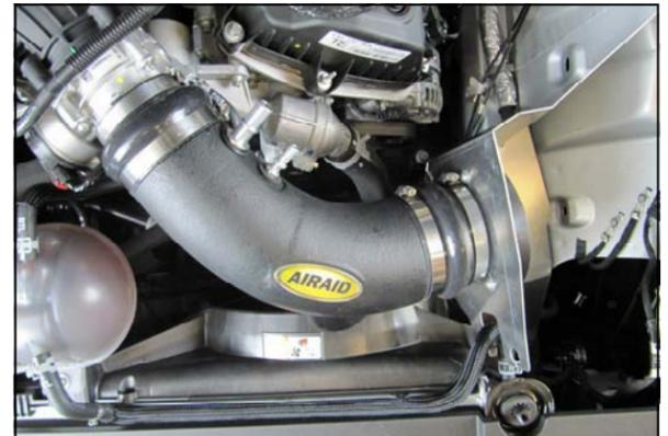
15. Install the Airaid Tube into the Hump Hose and Reducer as shown. Tighten all four Hose Clamps at this time.
