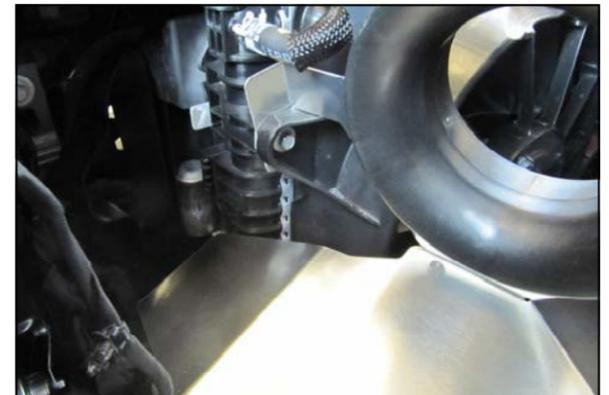
12 When properly installed, the Panel tab resides behind the fan shroud as shown.
