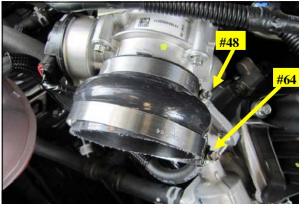
14. Slide the Reducer with one #64 and one #48 clamp onto the throttle body as shown.
