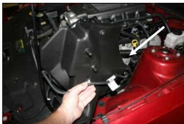
**5.** Turn the CAB so that the bottom faces the left fender as shown. Now reinstall the wiring loom anchors into their respective holes starting at the back of the CAB with the two hole anchor and work your way underneath and towards the front. The last anchor nearest the MAF sensor is not anchored.
