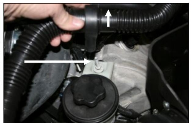
**9.** Lift up on the intake resonator tube to disengage it from the stud securing the power steering reservoir. Using a deep 10mm socket, remove the stud and save it for a possible optional install. See step #18.
