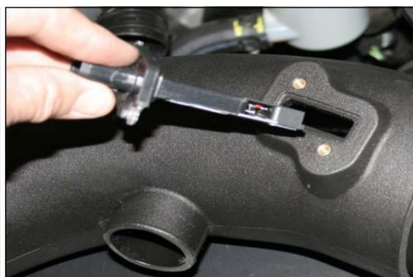
**8.** Install the MAF sensor into the intake tube using two provided 8-32x3/8" screws (#12). **Do Not Use The Factory Screws!**
