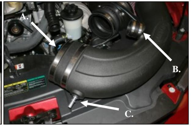
12.A.) Install the oval coupler onto the intake tube using two #72 hose clamps (#15). Leave the clamps loose for now. B.) Install the 1 3/4" coupler (#6) onto the intake tube using two #28 hose clamps (#16) as shown. Tighten *only* the clamp against the tube for now. C.) Install the provided grommet (#17) into the intake tube and then install the aluminum fitting (#20) into the grommet as shown.
