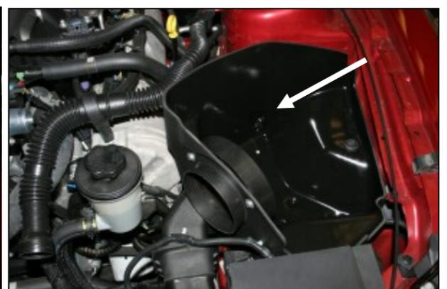
**6.** Install the CAB into the vehicle making sure that the scoop provision in the CAB aligns with the factory scoop, and the two locating pins on the bottom align with the factory grommets. Next reinstall the factory bolt that was removed in step #2 thru the steel sleeve and grommet and into the inner fender. Make sure that the wiring harness is not pinched under the CAB.
