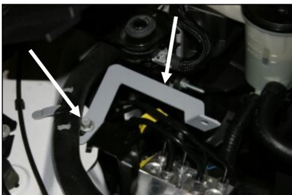
7. Lift up the corner of the plastic trim from step #6 to gain access to the bolt that secures the bracket for the anti lock brake manifold. Remove the bolt and install the front bracket (#17) as shown. Replace the factory bolt and leave it just snug for now.
