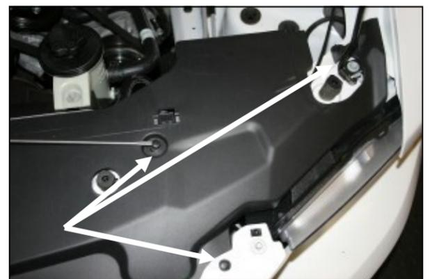
6. Using a flat blade screwdriver, pry up the center of the three plastic trim anchors that are shown. Once the center is up, then pry up the bottom half of the anchors up and out of the hole and save them for reinstallation in step #10.
