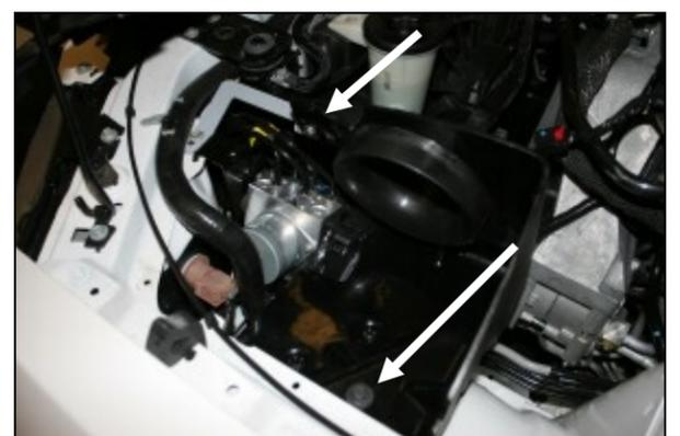
9. Install the CAD into the vehicle aligning the locating pins on the bottom of the CAD into the factory grommets in the fender. Reinstall the factory bolt from step #2 into the steel sleeve and grommet. Next install the 1/4-20x5/8" hex bolt (#14) thru one 1/4" flat washer (#9), thru the CAD, and thru the bracket securing it with one 1/4" serrated nut (#15). Adjust for fit and then tighten the bolt on the anti lock brake bracket.
