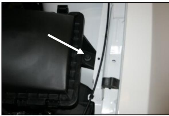
2. Remove the bolt that holds the factory airbox to the driver's side inner fender. (Save this bolt for later use in step #9).
