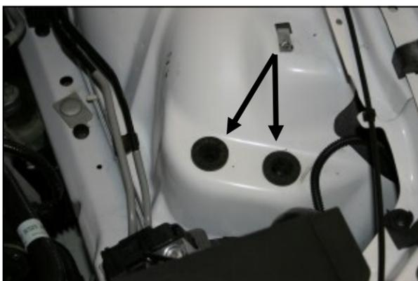
4. Make sure that you retain the factory grommets in the inner fender from the bottom of the factory airbox.
