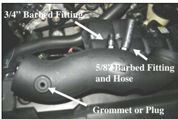
7. If your vehicle is equipped with an intake temp sensor (1999-01), install the supplied grommet (#17) into the hole in the Airaid Intake Tube (#2). On later models (2002-04), install the grommet plug (#18). Next install the two barbed fittings (#19 & #20) into the tube as shown. Now install the 5/8" x 3" hose (#16) onto the 5/8" barbed fitting.
