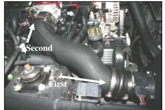
**12.** Install the Airaid Intake Tube into the hump hose first, and then onto the throttlebody. Adjust for fit, and then tighten the two remaining hose clamps. Reconnect the crankcase breather hose to the 5/8"x 3" hose, and connect the idle bypass hose to the 3/4" barbed fitting. Now reinstall the MAF sensor onto the MAF housing using the factory screws.
