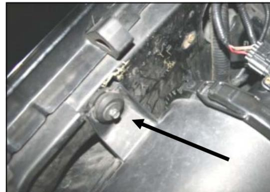
3. Remove the bolt that holds the factory air filter canister to the inner fender. Next remove the factory air intake tube from the throttlebody, and then the MAF housing. Now with a twisting motion remove the factory air filter canister from the vehicle.
