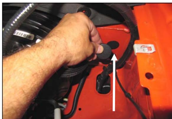
5. Plug the resonator hole in the firewall with the Firewall Plug (#15).
