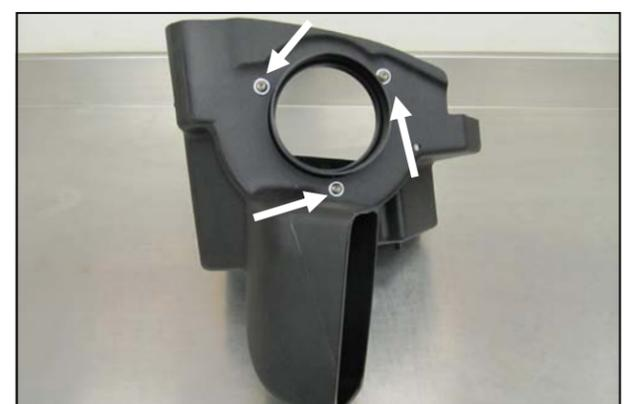
9. Install the Filter Adapter (#7) onto the Airaid Cool Air Box (#4) as shown. Use the three 1/4-20 button head bolts (#9), and flat washers (#10) to secure the Adapter.
