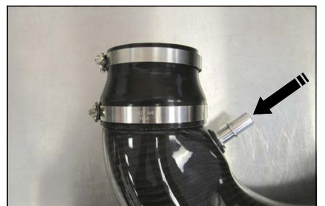
6. A.) Install the Silicone Reducer (#6) and Hose clamps onto the Airaid Intake Tube (#2). Place the #56 clamp (#14) on the Throttle body side of the reducer, and the #64 clamp (#13) on to the tube side. B.) Insert the 5/8" Grommet (#17) into the Intake tube as shown. Complete the tube assembly by inserting the 5/8 Aluminum Fitting (#16) into the Grommet.
