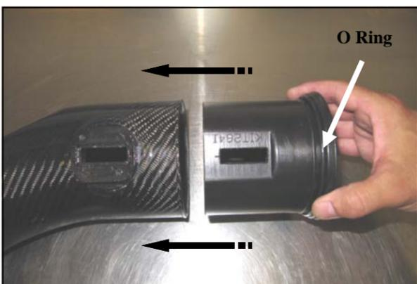
7. Slide the Modular Venturi Tube (#3) into the Airaid Intake tube (#2). Make sure to align the two slots for the Mass Air Flow sensor and that the O Ring (#18) is in Place.
