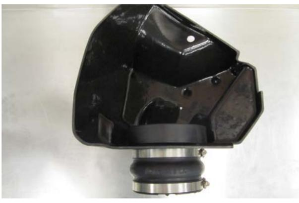
11. Install the hump hose (#5) and two #72 hose clamps (#12) onto the filter adapter as shown. Leave the two hose clamps loose for now.
