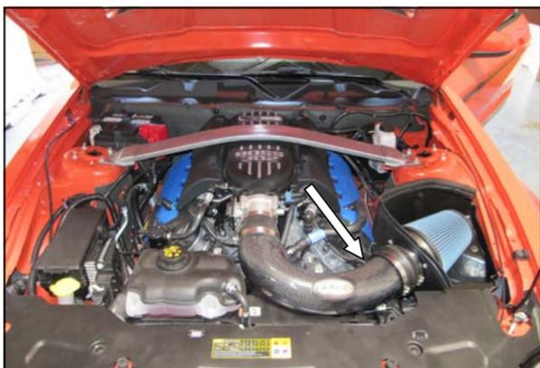
16. Reconnect the Mass Air Flow sensor, which is now located in the lower back side of the intake. Slide the locking tab back into the connector. Apply the Airaid Bubble Decal onto the Intake Tube as shown.
