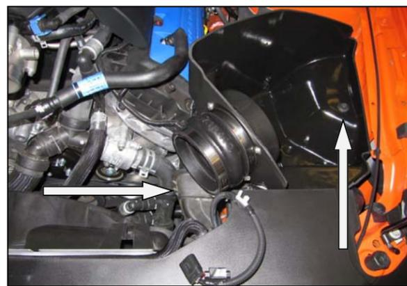
12. Install the CAB into the vehicle. Make sure that the air inlet of the CAB aligns with the factory duct, and the two locating pins on the bottom are seated in the factory grommets. Next reinstall the factory bolt that was removed in step #3 thru the steel sleeve and grommet and into the inner fender.
