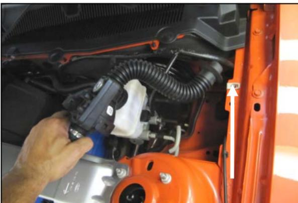
4. Unbolt the Intake resonator from the inner fender and disconnect it at the drivers side firewall. Remove the entire assembly from the vehicle and set it aside. It will not be reused.
