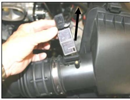
5. Using the provided #20 torx bit, remove two screws and the mass air sensor from the factory airbox lid. Note the direction of the sensor for proper re-installation later. (Save the mass air sensor for re-installation in step #13, the factory screws will not be re-used).
