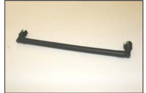
18. Install the 3/8"x12" hose (#8) onto the factory breather ends as shown.
