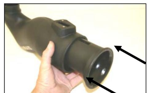
12. Install the Modular Venturi Tube (MVT) (#3) into the Airaid Intake Tube (#2) as shown. (SEE #22 BELOW!!)
