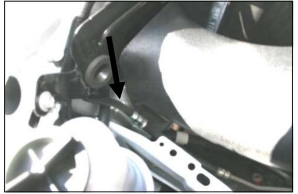
9. Due to inconsistent factory tolerances, some minor adjustment may be necessary to the factory A/C line so it will clear the Airaid MIT near the radiator support.. When all adjustments have been completed, tighten the nut, and button head bolt at the L-bracket.
