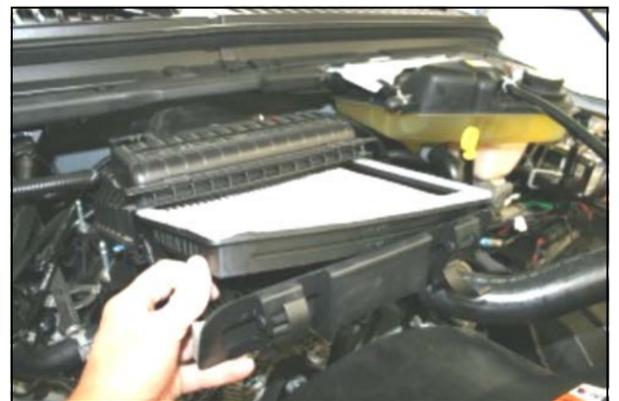
6. Install the Airaid Premium Filter (#1) into the factory airbox tray, slide it back in, and re-latch the two clips.
