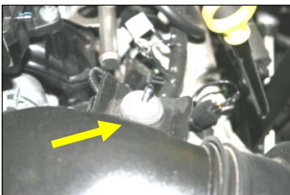
1. **Disconnect the negative battery cable.** With a 10mm wrench or deep socket, remove the nut from the stud that holds the factory intake tube to the mounting bracket. Save the nut for re-use later in the install.
