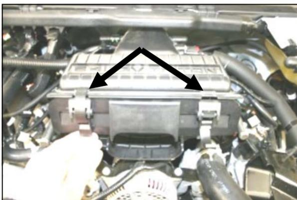
4. Unclip the two latches that hold the air cleaner tray into the air cleaner.
