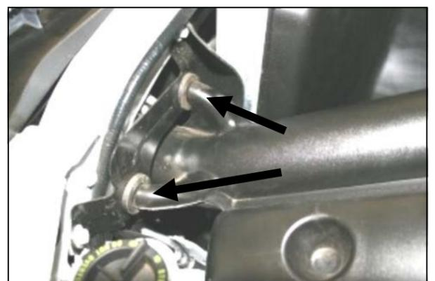
3. Remove the factory tube from the radiator support by pulling the tube out of the grommets. There are no bolts holding the tube. Remove the factory tube from the vehicle.
