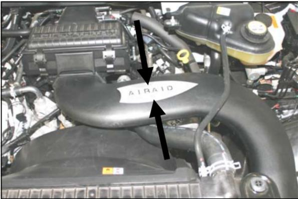
10. Install the Logo Plate onto the Intake Tube as shown, using the two Button Head Screws.
