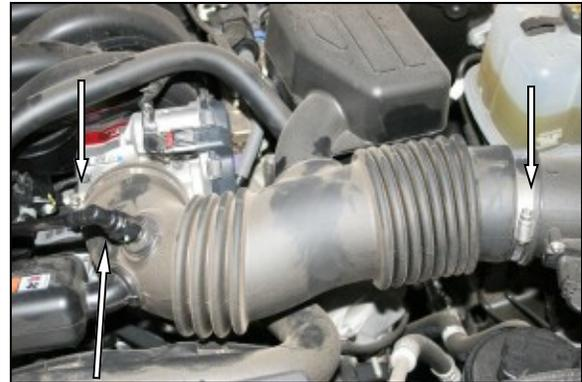
4. Re-install the factory intake tube onto the throttle body and the airbox lid, and tighten the hose clamps. Re-connect the breather hose to the factory intake tube. **Re-connect the negative battery cable!**
