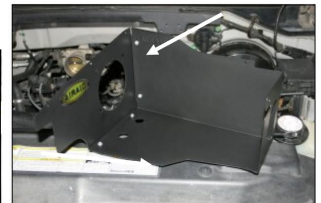
6. Assemble the MAF panel (#3), and bottom panel (#4) as shown using four 6-32 screws (#12), four flat washers (#13), and four Kep nuts (#14) as shown. Apply the Airaid Foil Decal onto the Panel as shown.
