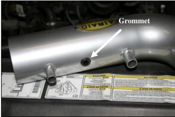
**13.** Install the supplied rubber grommet (#24) into the Airaid Intake Tube (#2) as shown. Apply the Airaid Decal onto the Intake Tube as shown.
