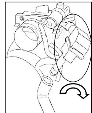
**15. 4.6L engines:** The idle air bypass line goes directly to the throttle body. Rotate the resonator box 90 degrees to provide clearance for the 3/4 x 12" L-hose (#7). Install the 3/4"x12" L-hose (#10) onto the Airaid Intake tube and the resonator box and secure it using the two #22 speed clamps (#23).
