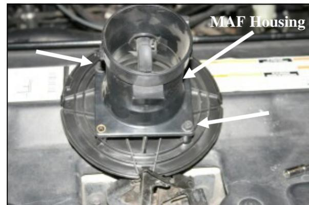
5. Remove the bolts that secure the MAF sensor housing to the adapter. Separate the adapter plate from the MAF sensor housing and save the sensor and housing for reinstallation in step #7.
