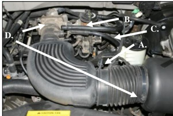
2. **A) Very carefully**, using a pulling circular motion, remove the air intake temperature sensor from the air intake tube. **B)** Disconnect the upper, idle air bypass hose. **C)** Disconnect the crankcase breather at the intake tube and the valve cover, and remove it from the vehicle. **D)** Loosen two hose clamps and remove the air intake tube from the vehicle.
