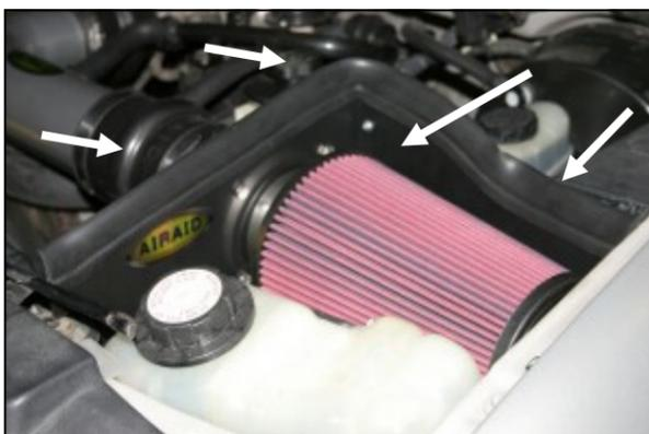
**16.** Reinstall the beauty cover using the 3 factory bolts. Install the Airaid Premium Filter (#1) as shown, and tighten the hose clamp. *If your vehicle does not have a hood mat, skip to Step #17.* Install the weatherstrip (#11) onto the top of the CAD as shown.
