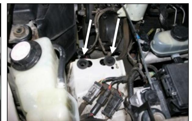
9. Remove the two grommets that held the air filter canister in place. They will not be reused.
