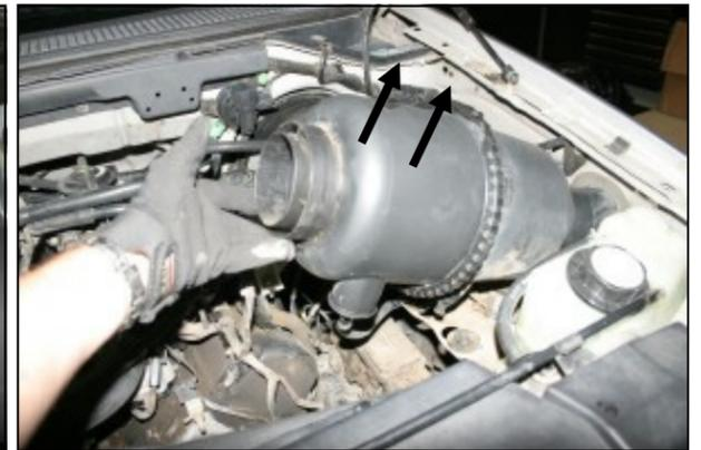
3. Lift straight up on the outlet side of the air filter canister to remove it from its locating grommets. Next, pull it towards the engine to dislodge it from the inner fender well.
