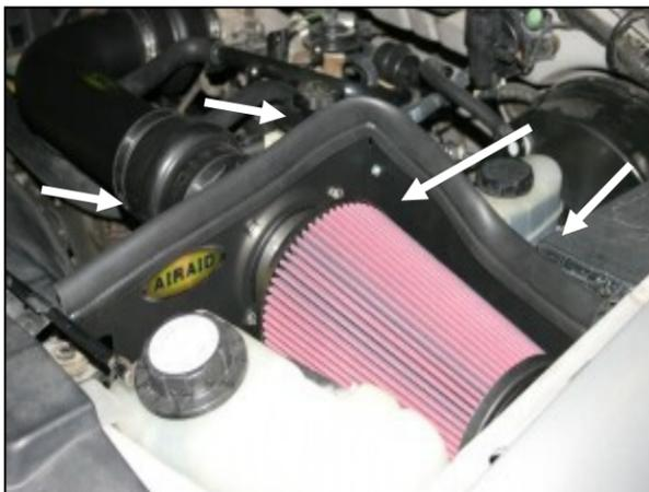
**16.** Reinstall the beauty cover using the 3 factory bolts. Install the Airaid Premium Filter (#1) as shown, and tighten the hose clamp. *If your vehicle does not have a hood mat, skip to Step #17.* Install the weatherstrip (#11) onto the top of the CAD as shown.
