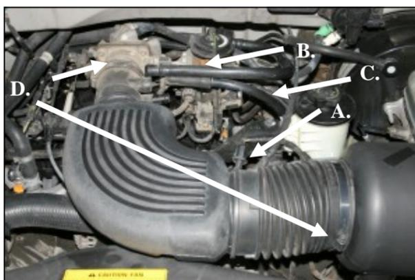
2. **A) Very carefully**, using a pulling circular motion, remove the air intake temperature sensor from the air intake tube. **B)** Disconnect the upper hard plastic tube from the air intake tube. **C)** Disconnect the crankcase breather at the intake tube and the valve cover, and remove it from the vehicle. **D)** Loosen two hose clamps and remove the air intake tube from the vehicle.
