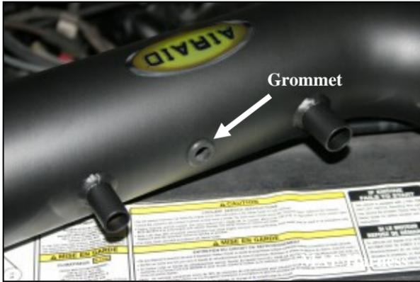
**13.** Install the supplied rubber grommet (#24) into the Airaid Intake Tube (#2). Apply the Airaid Decal onto the Intake Tube as shown.
