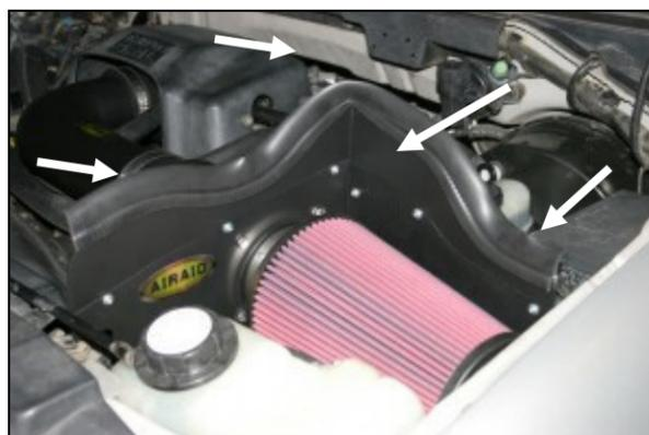
**17.** If your vehicle does not have a hood mat install the optional CAD height extender (#5) using five 6-32 screws (#12), flat washers (#13), and kep nuts (#14) as shown. Install the weatherstrip (#11) onto the top of the CAD as shown.
