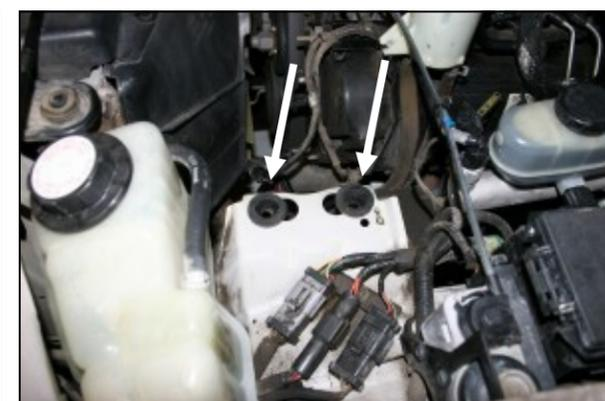
9. Remove the two grommets that held the air filter canister in place. They will not be reused.
