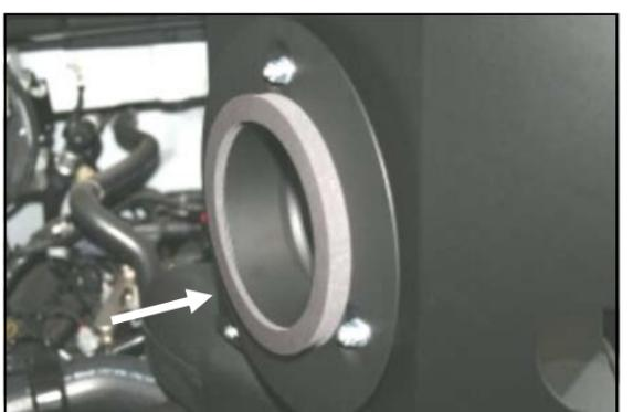
**7.** Install the gasket (#16) onto the filter adapter.
