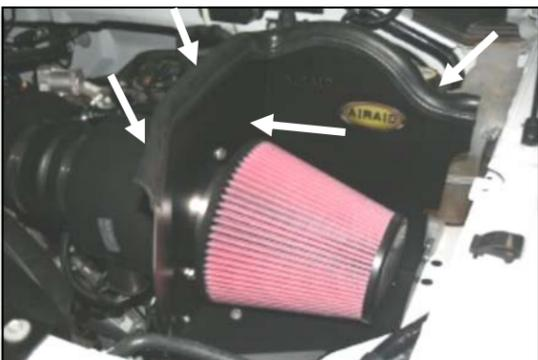
**16.** Install the Airaid Premium Filter (#1) onto the CAD and tighten the clamp. Install the weather strip (#8) onto the top edge of the CAD as shown. (Hint: start at one end and work your way around to the other.)
