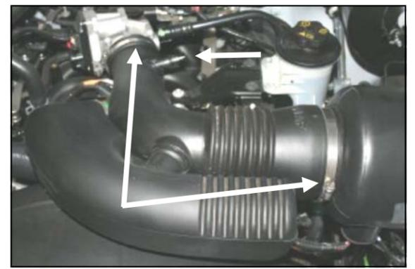
**3.** Slide the green tab on the factory breather hose, and remove it from the factory intake tube. Using a 5/16" socket, loosen the hose clamps on each end of the factory intake tube and remove it from the engine.
