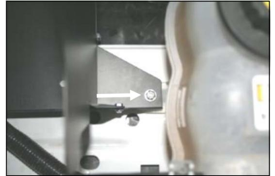
**12.** Align the hole in the CAD with the hole in the factory coolant reservoir mount. Insert one M6-1x25 hex bolt (#18) and 1/4" flat washer (#13) through the hole in the CAD, through the coolant reservoir mount, and into the speed nut below it.
