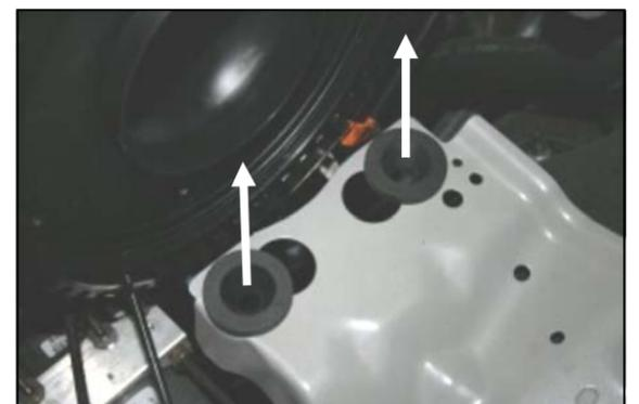
**9.** Remove the two factory grommets from the factory airbox mounting plate.
