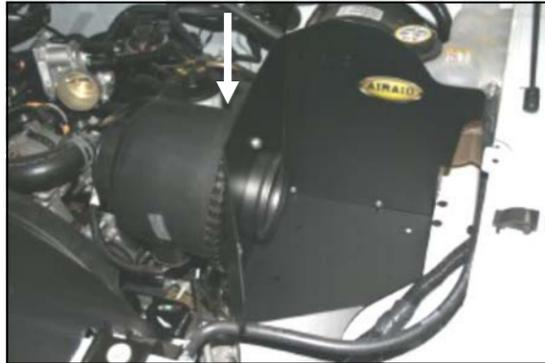
**11.** Install the CAD assembly into the vehicle. First, align the filter adapter with the factory MAF sensor housing, then, secure it with the factory clamp.
