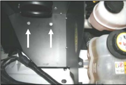
**13.** Insert two 1/4 - 20 x 7/8" bolts (#12) and 1/4" flat washers (#13) through the holes in the CAD and thru the grommets. On the underside of the factory airbox mounting plate, align the long/narrow bracket (#19), two 1/4" flat washers (#13), and two 1/4 - 20 locknuts (#15) with the 1/4-20 x 7/8" bolts. Tighten the assembly securely.
