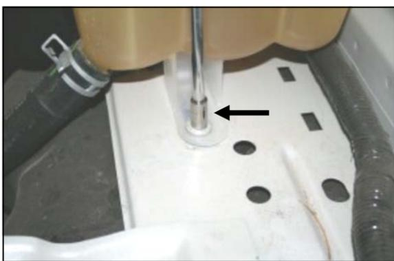
**4.** Using a 5/16" socket, ratchet and extension, remove one bolt from the factory coolant reservoir mount.
