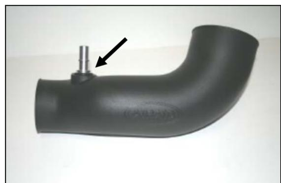
**8.** Install the rubber grommet (#22), and aluminum fitting (#21) into the Airaid Intake Tube (#4).
