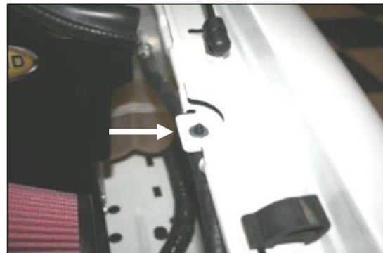
**17.** Slip the black plastic hose mount (#20) over the radiator overflow hose. Next, place one 1/4" flat washer (#13) over the hole on the inner drivers side fender. Slide the hose mount prongs thru the fender and thru the washer.
