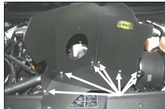
**5.** Assemble the Airaid Cool Air Dam (CAD) panels (#2, #3) using seven 6-32 x 5/16" screws (#9), #6 flat washers (#10), and 6-32 keps nuts (#11). Apply the Airaid Foil Decal onto the Panel as shown.
