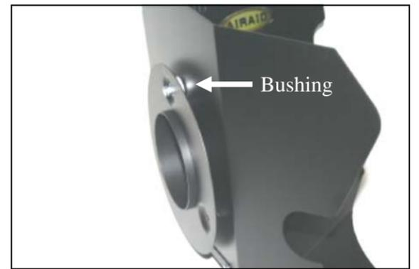
**6.** Insert three 1/4-20 x 7/8" bolts (#12), and 1/4" flat washers (#13) through the CAD. Place one bushing (#14) at each hole between the CAD and the filter adapter (#5). Next, secure the assembly using three 1/4" flat washers (#13), and 1/4-20 locknuts (#15).
