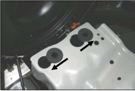
**10.** Slip two rubber grommets (#17) into the large holes in the factory airbox mounting plate, and then slide them sideways into the small holes as shown.
