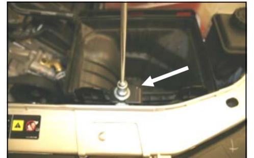
**6.** With a 10mm socket, remove and save the bolt that holds the factory air filter base to the radiator support. Remove the air filter base from the vehicle.
