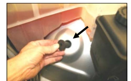
**9.** Slip the well nut (#22) into the hole in the inner fender.
