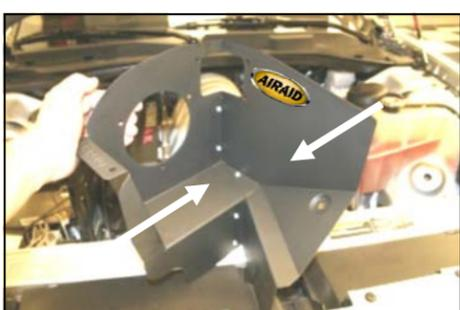
**7.** Assemble the two Cool Air Dam (CAD) panels (#2, #3) using five 6-32 x 5/16" screws (#16), #6 flat washers (#17), and 6-32 keps nuts (#18). Apply the Airaid Decal on the Panel as shown.
