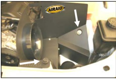
**10.** Install the CAD into the vehicle. Re-install the factory bolt removed in step #6 thru the CAD and into the radiator support. Next install the 3/8-16 x 1 1/4" button head bolt (#11) and 3/8" flat washer (#12) thru the CAD and into the well nut. Tighten both bolts.
