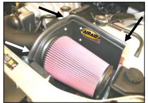
**18.** Install the Airaid Premium Filter (#1), onto the filter adapter inside of the CAD, and tighten the hose clamp. Next install the weather strip (#10) onto the top of the CAD.
