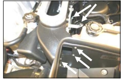
12. Install the hood scoop into the CAD using three 8-32 x 3/8" button head screws (#14), and three #8 flat washers (#15), leave loose. Install the L-bracket (#23) over the stud on the fender, and bolt it to the hood scoop using one 1/4-20 button head bolt (#12), and 1/4" flat washer (#13). Replace the factory nut on the stud, adjust for fit, and tighten all bolts, nuts, and
