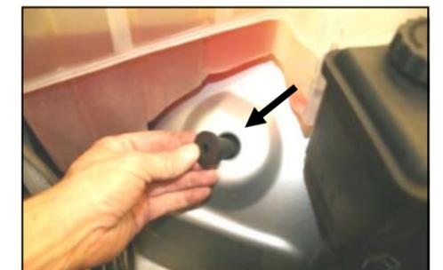
**9. Slip the well nut (#22) into the hole in the inner fender.**
