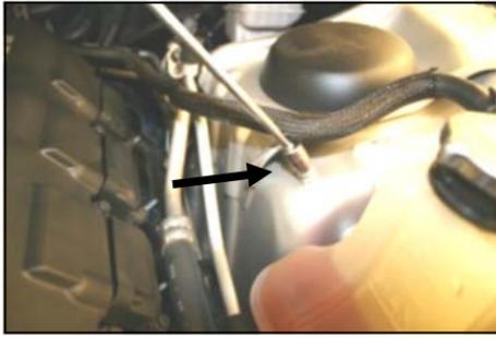
11. Remove the factory 10mm nut from the stud on the driver's side inner fender and save it for the next step.
