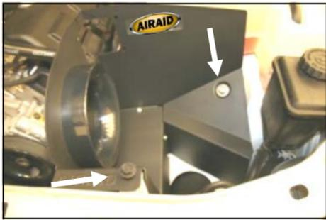
10. Install the assembled Cool Air Dam into the vehicle. Re-install the factory bolt removed in step #6 thru the CAD and into the radiator support. Next install the 3/8-16 x 1 1/4" button head bolt (#10) and 3/8" flat washer (#11) thru the CAD and into the well nut. Tighten both bolts.
