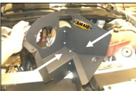
**7. Assemble the Airaid Cool Air Dam (CAD) panels (#2, #3) using five 6-32 x 5/16" screws (#16), #6 flat washers (#17), and 6-32 keps nuts (#18). Apply the Airaid Foil Decal onto the Panel as shown.**
