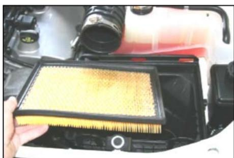
**4.** Remove the factory air filter from the bottom of the airbox.
