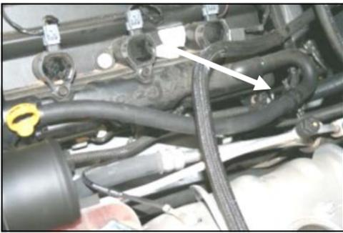
**10. For 2.7L Engines:** After installing the Quick Fit Panels, (Refer to step #7), connect the breather hose to the factory elbow at the back of the valve cover using one #16 speed clamp. (Factory intake tube removed for instruction purposes).
