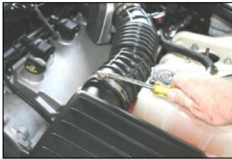
**2.** Loosen the hose clamp on the factory intake tube, located at the air box lid.
