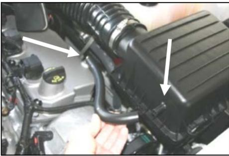
**1. Disconnect the negative battery cable.** Remove the breather hose from the factory air box lid and valve cover.
