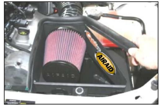
**12.** Install the weather strip (#4) on the top of the Quick Fit panels. (Hint: Start at one end and work all the way to the other end).
