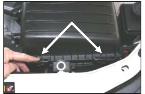
**3.** Remove the airbox lid by pulling the tabs towards the front of the car. Then, lift the lid up and slide it forward, and remove it from the bottom of the airbox.
