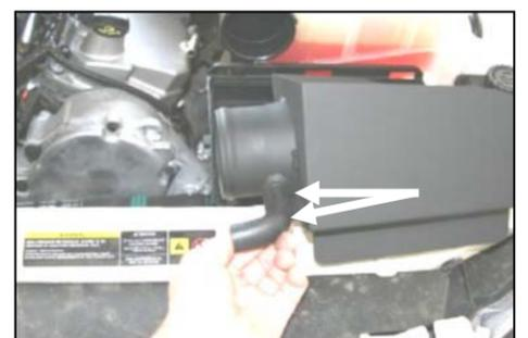
**6.** Slide the 1/2" rubber elbow (#8) onto the breather fitting on the side of the Quick Fit panels. Install 2 #18 speed clamps (#9), one over each end of the elbow, (*Do not tighten the clamps at this time.*)
