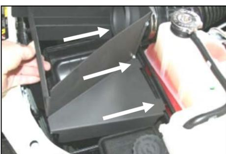
**7.** Slide the three tabs on the back of the Quick Fit panels into the factory airbox. (*For 2005-2006 models, make sure the 1/2" rubber elbow (#8) slides onto the valve cover breather nipple.*) Push the front of the Quick Fit panels down, until the locking tabs snap into place. **2.7L Engines:** Skip to step #9.
