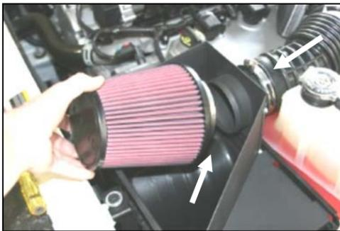
**11.** Slide the Airaid Premium Filter (#1) onto the Quick Fit panel tube, and tighten the hose clamp. Install the factory intake tube onto the opposite end of the Quick Fit panel tube, and tighten the hose clamp. Tighten the speed clamps on the breather hose, and the 1/2" rubber elbow.
