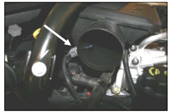
6. Disconnect the intake air temperature sensor wiring harness, by squeezing the tab on the side, and sliding the connector off.
