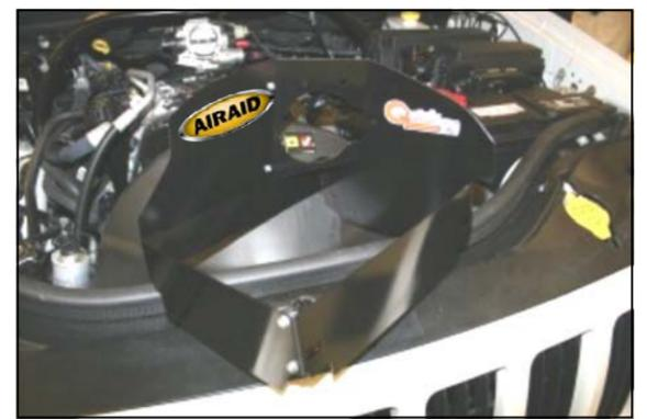
9. Assemble the Quick Fit panels as shown, using five 6-32 screws (#16), #6 washers (#17), and keps nuts (#18). Apply the Airaid Foil Decal onto the Panel as shown.
