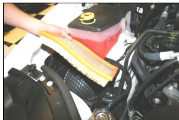
5. Remove the factory air filter.
