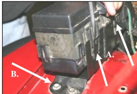
8. A.) On the right fender, pry two tabs away from the fuse box, lift it up and set it off to the side. B.) Next, remove and save the outside bolt from the fuse box mount.
