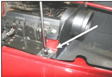
14. Re-install the factory bolt from step # 8 thru the CAD, and into the fender. Re-install the fuse box on the factory mount.
