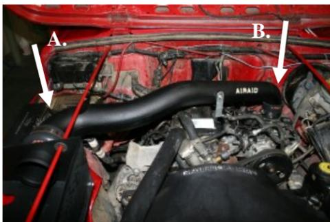
19. A.) Install the large end of the Airaid Intake Tube into the hump hose.
