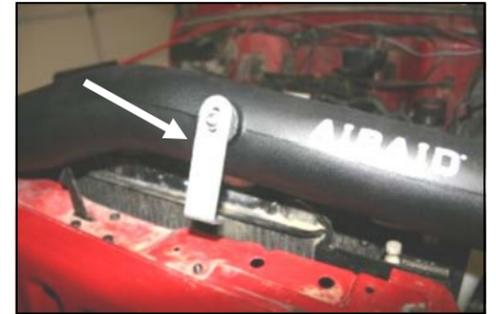
18. Install the L-bracket (#18), onto the Airaid Intake Tube (#4), using one 1/4" button head bolt (#11), and flat washer (#12). Leave the bolt loose for now.
