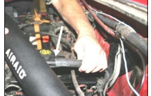
21. Re-connect the breather hose to the Airaid Intake Tube.
