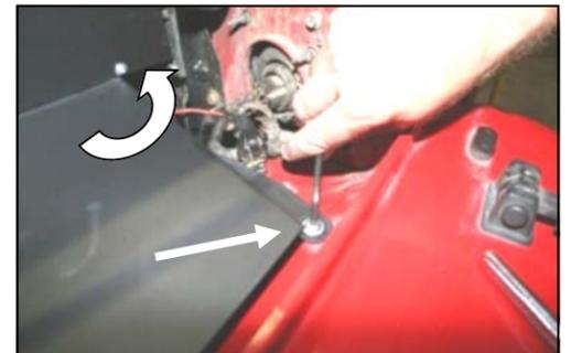
15. Install the supplied 1/4" button head bolt (#11), and 1/4" washer (#12), thru the CAD, with the 1/4" fender washer (#13) and nut (#14), on the bottom of the fender. Re-install the factory bolt in the radiator shroud removed in step #9.
