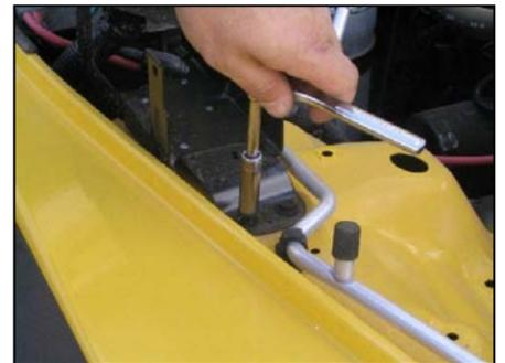
**8.** Using a 10mm socket, remove one bolt from the inner fender as shown above. Retain bolt for later use.
