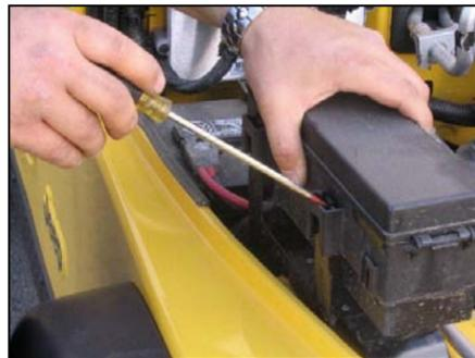
**7.** Using a flat blade screwdriver, push locking tabs inward to remove the fuse panel from the mounting bracket. Position panel out of the way to access the bolt underneath.
