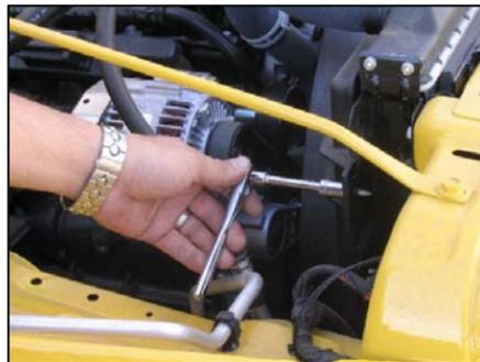
**6.** Using a 7/16" socket, remove the factory radiator mount bolt. Retain bolt for later use.
