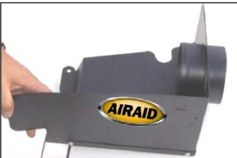
**10.** Using the supplied hardware, assemble the Airaid Cool Air Dam assembly as shown above. Apply the Airaid Decal as shown, on
