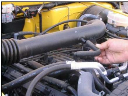
**1.** Disconnect negative battery cable. Remove factory valve cover breather hose from intake tube and discard. Retain plastic valve cover fitting for later use.
