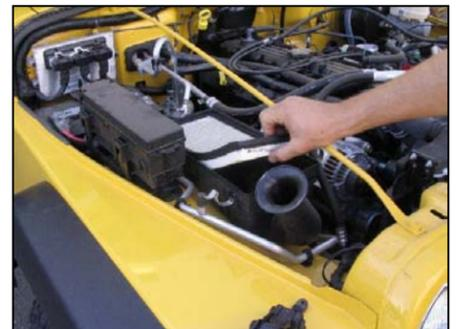
**4.** Remove factory air filter from airbox.
