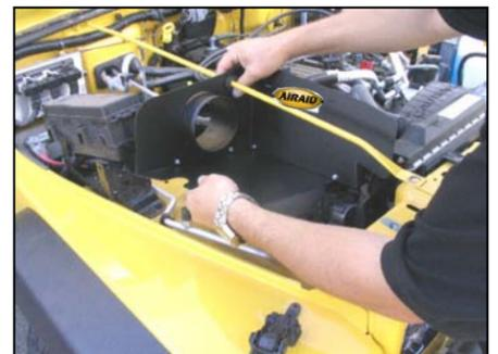
**12.** Carefully slide the Airaid Cool Air Dam assembly over the passenger side radiator support rod. Be careful not to scratch the paint. Insert the rubber grommet into the panel for final positioning of the assembly.
