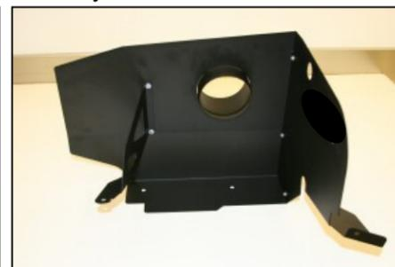
**7.** Assemble the Cool Air Dam as shown using the 5 screws, washers, and nuts provided.
