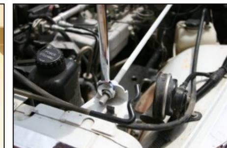
**8.** Using a 9/16" wrench, loosen the nut on the radiator rod support, and lift it up.
