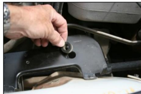
**4.** Remove the two grommets from the airbox mounting plate.
