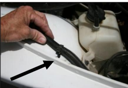
**6.** Carefully remove wire loom clamp from hole in fender.
