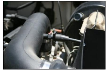
16. Slide intake tube into the hump hose first, and then into the coupler. Adjust for a good fit, and tighten hose clamps. Slide vacuum hose on barbed fitting, and install speed clamp as shown.
