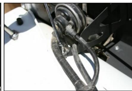
**11.** Slide the CAD bracket under the throttle body and reinstall the factory bolt from step 5.
