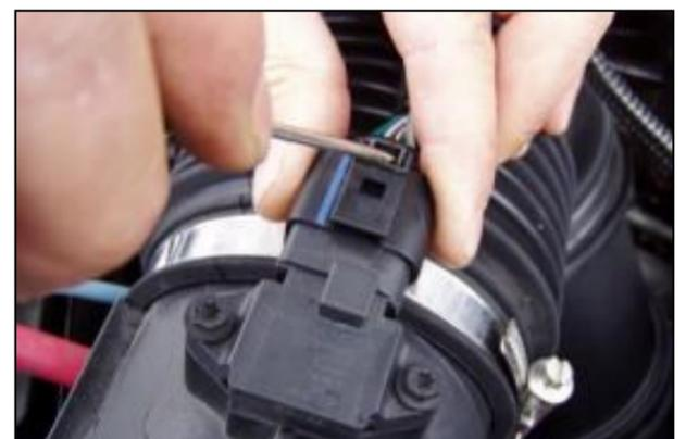
9. Re-connect the wire harness to the sensor on top of the adapter.
