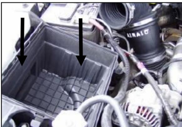
8. Install Airaid intake assembly in place of the factory air box lid & tighten factory hose clamp on intake tube to Airaid system.
