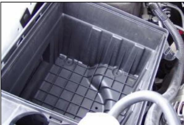
4. Loosen the clamp connecting the factory air box lid to the factory air intake tube and unclip the factory air box lid and remove entire filter/intake assembly from vehicle. (Note: leave the lower factory air box lid in place)
