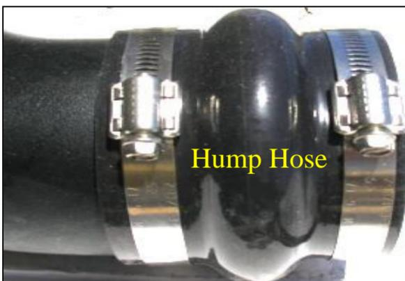
**8.** Slide the urethane hump hose onto straight end of Airaid intake tube with two #60 hose clamps. (*Note: Leave hose clamps loose until final assembly.*)
