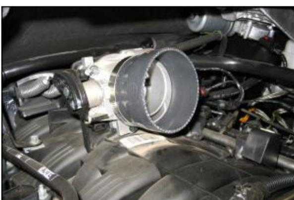
**7.** Install the reducer hose and a #52 hose clamp onto the throttle body. Install a #56 hose clamp onto the other side of the reducer.
