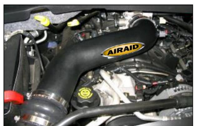
**9.** Install Airaid intake tube assembly by connecting the Airaid hump hose onto the factory air box lid and the other end onto the Airaid reducer hose. Tighten all hose clamps. Apply the Airaid Bubble Decal onto the Intake Tube as shown.
