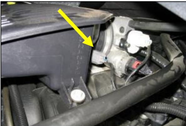
**4.** Disconnect the factory electrical connector from the factory air temperature sensor.
