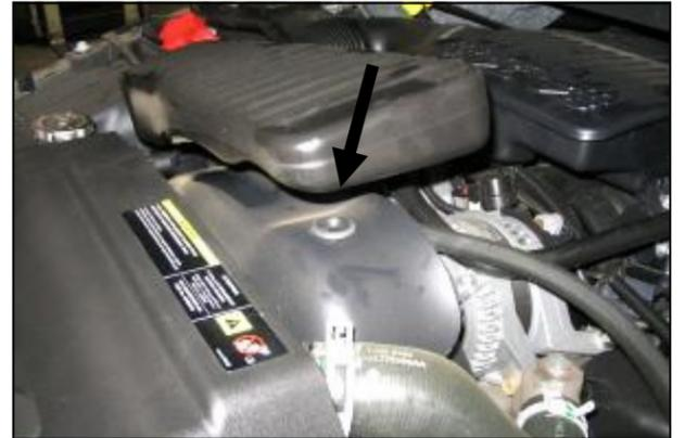
**3.** Unsnap the factory silencer box from the fan shroud and remove the factory tube assembly from the vehicle.
