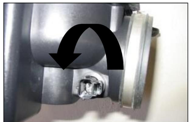
**6.** Turn the air temperature sensor 1/4 turn and remove from the air box. Retain sensor for later use.
