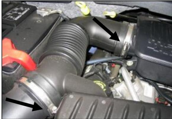
**2.** Loosen the two hose clamps on each end of the factory intake tube.
