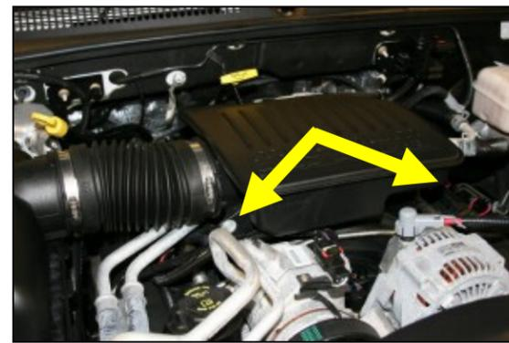
**3. With the 10mm socket, remove 2 bolts** from the base of the resonator.
