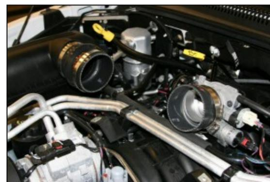
**6. Install the urethane hump hose** on the factory airbox with the two #60 hose clamps. (Leave clamps loose.) Next install the reducer (small side first with the #48 hose clamp) on the throttle body. Install the #52 hose clamp on the outside of the reducer, and leave loose.
