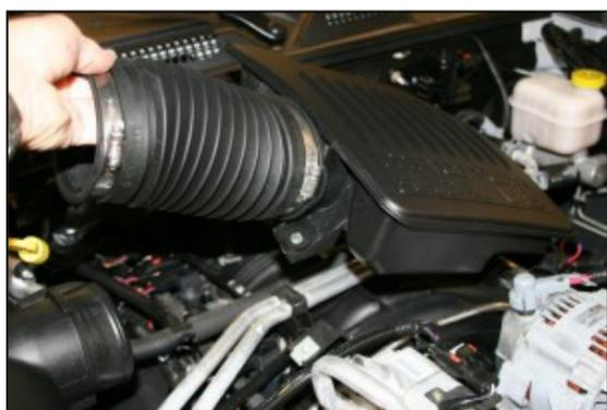
**4. Remove the resonator and tube** from the vehicle.
