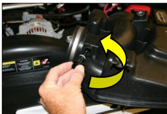
**5. With the resonator turned over, carefully remove the air temp sensor** by pushing in, and turning counter clockwise.
