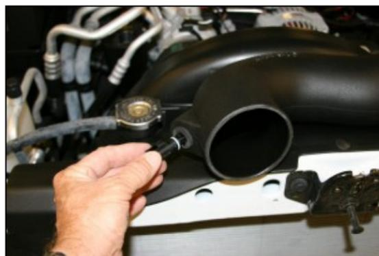
**8. Carefully install the air temp sensor** into the grommet installed in step 7. Make sure it goes all the way in.
