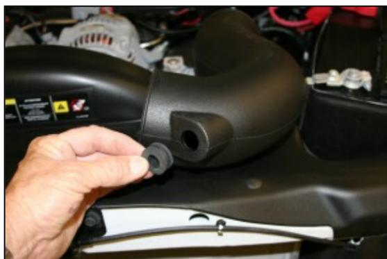
**7. Install the grommet** into the hole in the MIT as shown.
