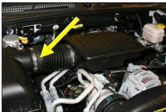
**1. Disconnect negative battery cable.** Loosen hose clamp on intake tube at the factory airbox end. For Jr. Kit, replace the factory air filter with the Airaid Premium Filter provided.
