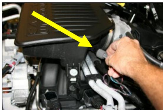
**2. Disconnect the intake air temperature sensor** by squeezing the tab on the connector.
