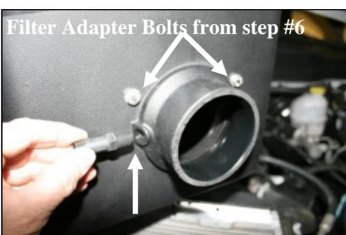
**7.** Install the 1/4" NPT x 1/2" Barbed fitting (#16) into the CAD as shown. **2002-03 Models** Install the 1/4" hex plug (#17) in place of the barbed fitting.
