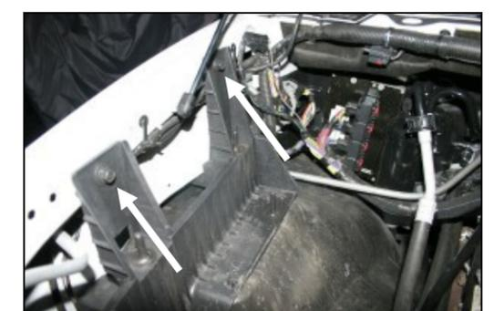
**9.** Remove the two bolts that secure the airbox mounting bracket to the inner fender. They will be reinstalled in step #10.
