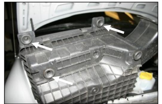
**3.** Turn the factory air box over and remove 3 of the 4 grommets. They will be reinstalled in the Airaid Cool Air Dam in step #8.
