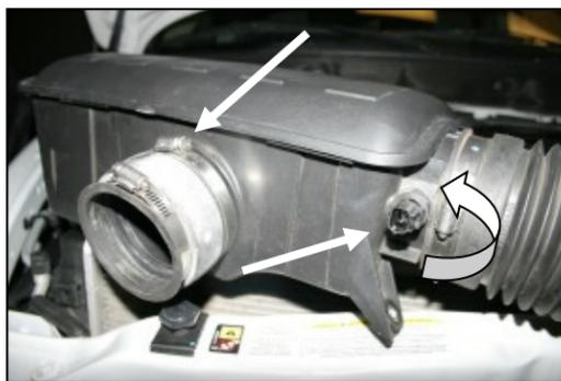
**5.** Loosen the factory hose clamp on the coupler and remove the coupler assembly from the resonator. **2003-07 Models** Next gently push in on the temperature sensor and rotate it to the left and remove it from the resonator. These parts will be reinstalled on the Airaid intake tube in step #12.
