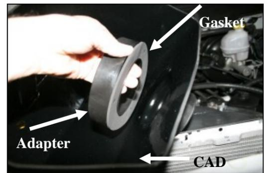
**6.** Install the filter gasket (#21) and filter adapter (#5) onto the Airaid Cool Air Dam (#3) as shown using three 1/4" x 5/8" bolts (#7), and 1/4" flat washers (#8). Refer to the line drawing above for reference.
