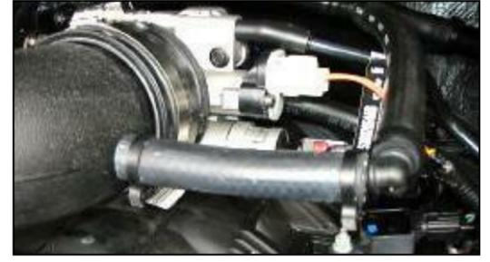
**15. 2002-03 Models;** Install one end of the provided 90° barbed fitting (#20) into the factory breather hose and then connect the supplied 1/2" breather hose (#19) to the other end. Connect the hose to the nipple on the Airaid intake tube. Secure all three connections with the provided #16 Speed Clamps (#15).
