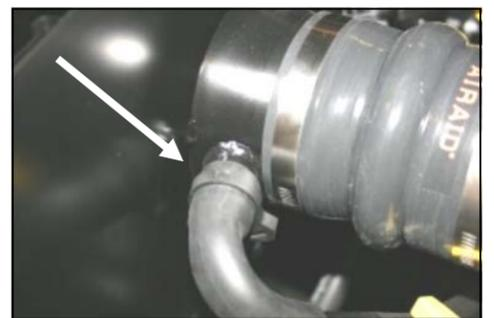
**12.** Install the provided #24 speed clamp (#9) over the hose onto the nipple on the CAD. Squeeze the clamp to secure the hose.
