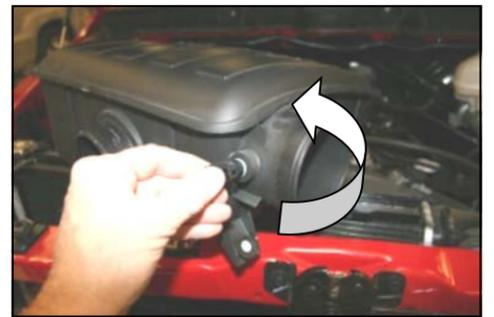
**6.** Gently twist the air temperature sensor counterclockwise and remove it from the resonator.
