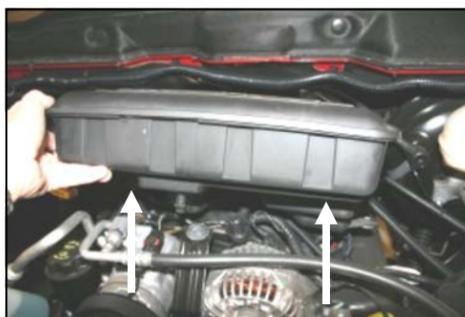
**5.** Lift the front of the resonator straight up, and then pull towards you to remove it from the vehicle.
