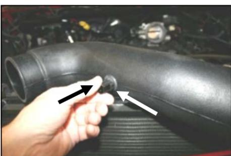
**7.** Install the supplied grommet (#10) into the Modular Intake Tube (#3). Next, carefully slide the factory temperature sensor into the grommet until it touches the tab on the temperature sensor.
