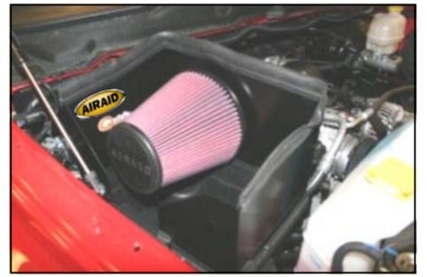
15. Install the Airaid Premium Filter (#1) onto the tube on the CAD and tighten the hose clamp. Next install the weather strip (#5) on the top of the CAD as shown. Apply the Airaid Foil Decal onto the Panel as shown.
