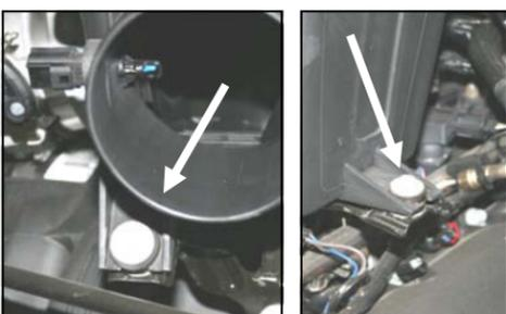
**4.** With a 10mm socket, remove two bolts holding the intake resonator to the intake manifold brackets.
