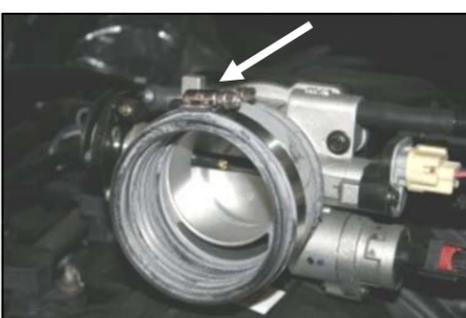
**10.** Install a #56 hose clamp (#6) on the factory throttle body coupler. Leave loose for now.
