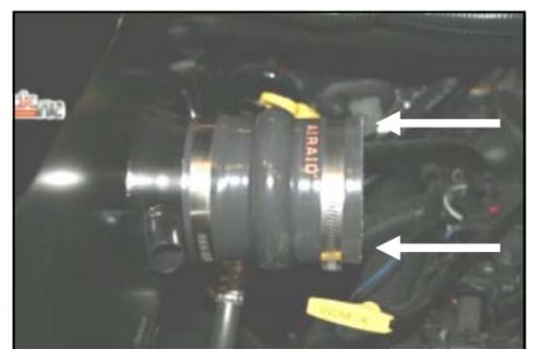
**9.** Install the urethane hump hose (#4) onto the tube on the CAD using two #60 hose clamps (#7). Leave clamps loose.
