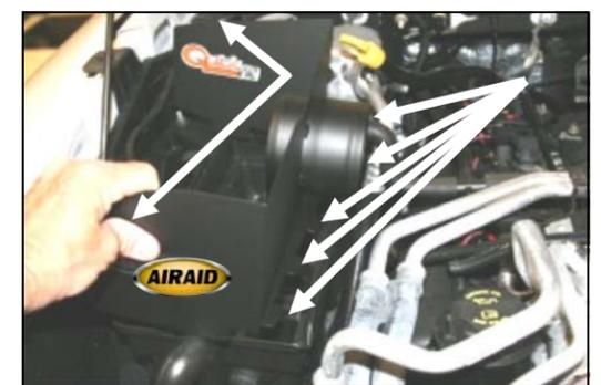
**6.** Slip the five tabs of the Quick fit panel (#2) through the slots on the airbox base. Adjust the panel for fit, then re-latch two of the factory clips onto the panel. Apply the Airaid Foil Decal onto the Panel as shown.
