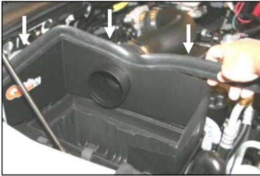
14. Install the weather strip (#6) onto the top of the Quick Fit Panel as shown. (Hint: Start at one end and work towards the other.)
