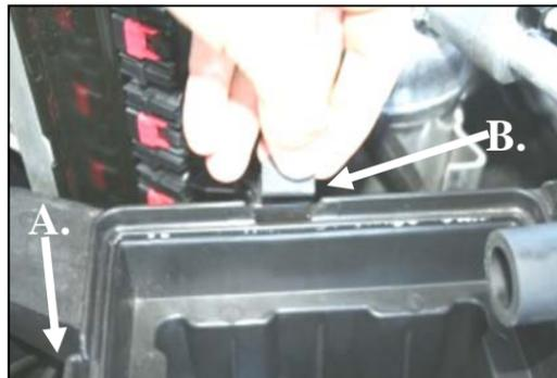
**5. 2007 Models only:** A.) Using a flat blade screwdriver, gently pry and remove one factory clip from the passenger side rear of the airbox base. (see arrow above)
