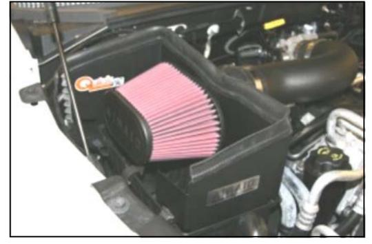
15. Install the Airaid Premium Filter (#1) onto the Quick Fit Panel as shown, and tighten the clamp.
