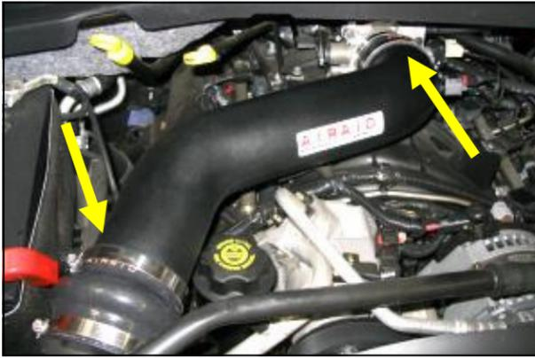
14. Install the Airaid intake tube assembly by connecting the Airaid hump hose onto the air filter adapter, and the other end into the Airaid reducing coupler. Tighten all hose clamps.
