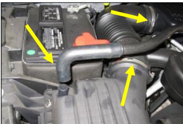
1. Disconnect the negative battery cable. Disconnect the breather hose from the factory air box lid. Loosen the two hose clamps on each end of the factory intake tube.
