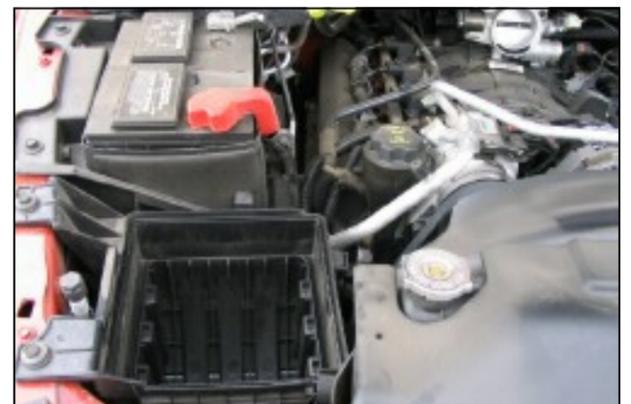
3. Unlatch the metal clips and remove the lid from air box base. Using a 13mm socket, remove the air box base from the engine compartment.
