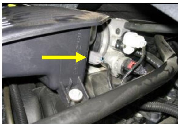
5. Disconnect the factory electrical connector from the factory air temperature sensor.
