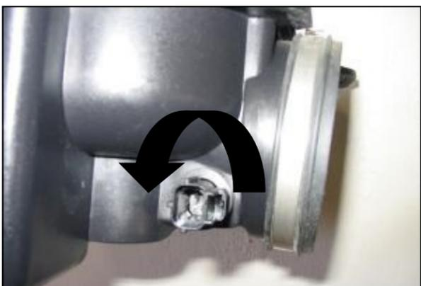
7. Turn the air temperature sensor 1/4 turn and remove from the air box. Retain sensor for later use.
