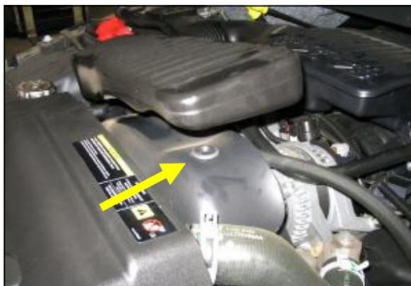
2. Unsnap the factory silencer box from the fan shroud and remove the factory tube assembly from the vehicle.
