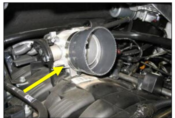
12. Install the supplied reducing coupler and #52 hose clamp onto the throttle body. Install the #56 hose clamp on the opposite end.
