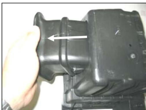
**4.** Using a flat blade screwdriver, carefully un-snap the air box base inlet from the air box base and remove it. Reinstall the factory air box base into the engine compartment without the inlet.
