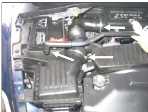
**1. Disconnect the negative battery cable.** Remove the valve cover breather hose from the factory air box lid. Loosen the hose clamps on both sides of the factory intake tube.
