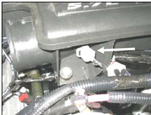
**5.** Carefully disconnect the factory air temperature sensor wiring harness from the sensor in the resonator.
