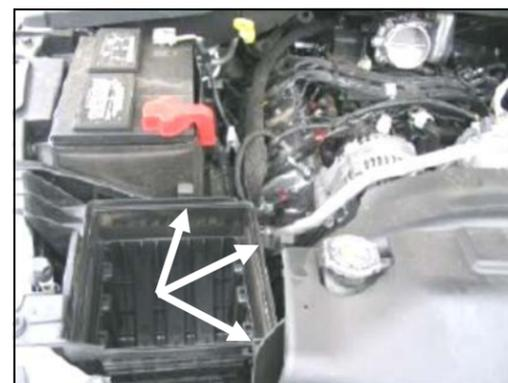
**3.** Unlatch the clips that secure the air box lid to the air box base, and remove the air box lid from the vehicle. Using a 13mm socket, remove the air box base from the engine compartment.
