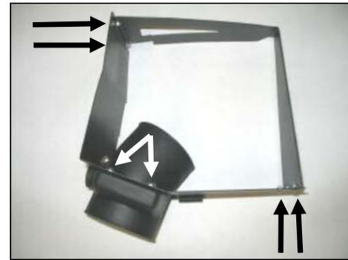
**9.** Assemble the Airaid Quick Fit Panels (#2, #3) using four 6-32x5/16" screws (#10), #6 flat washers (#11), and 6-32 keps nuts (#12). Next, install the air filter adapter (#4) using two 1/4-20x1/2" button head screws (#13) and 1/4" flat washers (#14).
