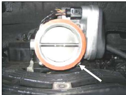
**8.** Remove the factory orange seal from the throttle body.
