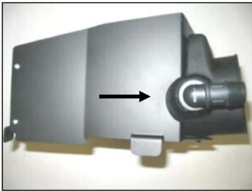
10. Install the nylon fitting (#15) into the air filter adapter as shown.
