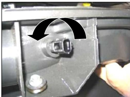
**7.** Remove the factory air temperature sensor from the resonator by turning it counter clockwise and pulling it straight out (save for reuse).
