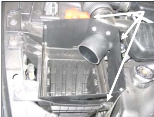
11. Install the Quick Fit Panels onto the top of the factory air box base. Relatch the factory clips onto the tabs on the Quick Fit Panels.
