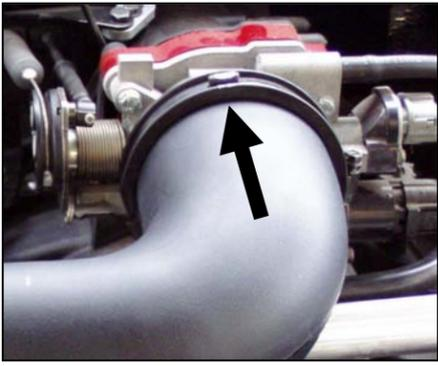
13. Factory coupler must be orientated with the clamp screw at the 12 o'clock position.
