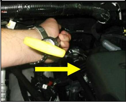
17. If your vehicle is equipped with a dipstick tube that interferes with the location of the Airaid Intake System, an adjustment to the dipstick tube must be made. Firmly grasp the dipstick tube about 6 inches below the top with your left hand and carefully form the tube towards the engine. This will allow for clearance of the Airaid Intake System.
