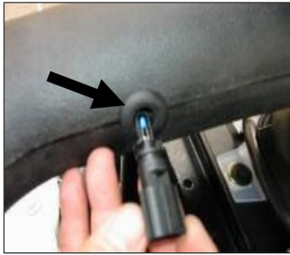
14. If your vehicle is equipped with an air temperature sensor, insert the rubber grommet into the hole on the intake tube and mount the air temperature sensor into the grommet.
