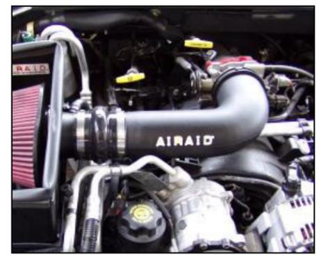
12. Slide the intake tube into the throttle body & align hump hose with Airaid Cool Air Dam. Slide the hump hose over end of the Airaid Cool Air Dam intake and secure using a #56 hose clamp.
