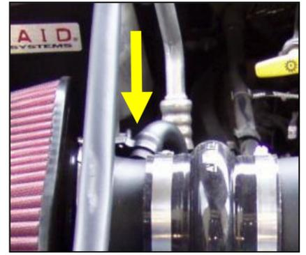
16. Reconnect the crankcase breather hose to the tube on the Airaid Cool Air Dam and secure with the black speed clamp provided. (Note for 2004: Replace breather hose with new 1/2" ID hose and speed clamps provided.)
