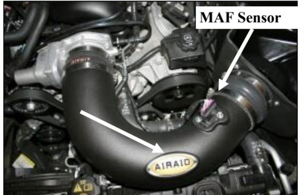
15. Install the Airaid Intake Tube into the hump hose first, and then into the reducing coupler. Adjust for fit, and tighten all four hose clamps. Next install the MAF sensor into the tube and secure it using two 8-32 x 3/8" button head screws. Apply the Airaid Decal onto the Intake Tube as shown.
