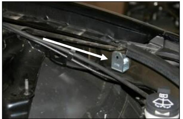
12. Replace the ground lug from step #11 with the ground bracket as shown using the 6mm hex bolt, and lock washer.
