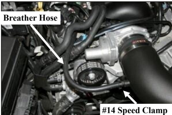
16. Install the 3/8" barbed fitting into the Airaid Intake Tube. Next install the 3/8"x18" breather hose between the barbed fitting and the steel crankcase breather tube on the rocker cover. Refer to step #2. Install one #14 speed clamp over the breather hose at the barbed fitting as shown.
