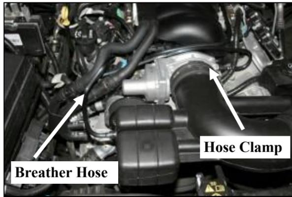
2. Pull the crankcase breather hose out of the air intake tube using a firm tug. An O-ring is all that keeps it attached to the tube. Push the small tab on the hard plastic crankcase breather hose on top of the passenger side valvecover to release it from the steel breather line. Remove it from the vehicle. Next loosen the hose clamp that secures the air intake tube to the throttle body.
