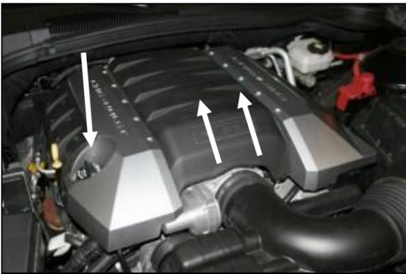
1. **Disconnect negative battery cable.** Remove the oil fill cap and then lift up on the front of the engine cover to remove it from the vehicle. Replace the oil cap for now to make sure nothing falls into the crankcase during the install.
