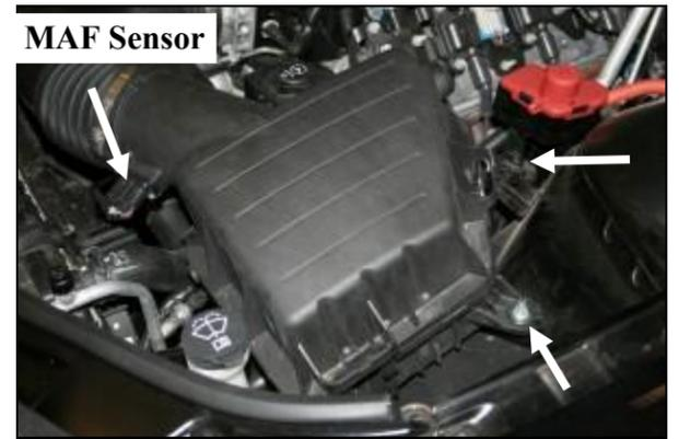
3. Using a deep 10mm socket, remove and save the two nuts that secure the factory airbox to the fender well. Using a 9/32" wrench or a #20 Torx bit, remove the two screws that secure the Mass Air Flow (MAF) sensor into the air intake tube. Without disconnecting the MAF, carefully remove it from the tube and set it out of the way on top of the engine.
