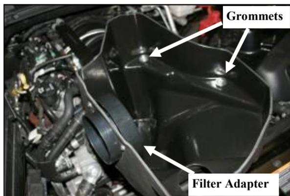
8. Reinstall the two steel sleeves and grommets into the Airaid Cold Air Box (CAB). Next install the filter adapter into the CAB as shown using three 1/4-20 button head bolts, and 1/4" flat washers. Refer to the line drawing above for details.
