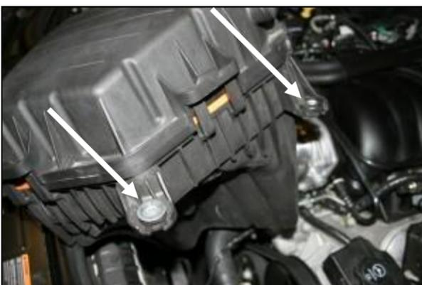
7. Remove the two steel inserts, and grommets from the factory airbox. Save these pieces, they will be reused in step #8.
