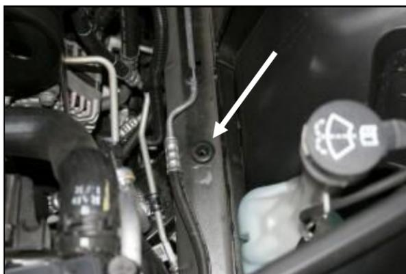
5. Use caution not to lose the factory grommet when you remove the air intake assembly. It will be needed if you ever want to reinstall the factory intake assembly.
