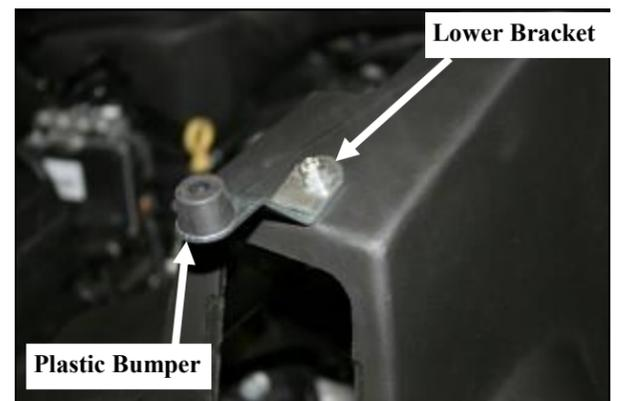
9. Turn the CAB upside down and mount the lower bracket to the bottom of the CAB using one 1/4-20x3/4" hex bolt, 1/4" flat washer, and 1/4" Nylock nut as shown. Next using one 8-32x5/8" button head screw, and one #8 Kep nut, attach the plastic bumper to the bracket as shown.
