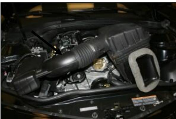
4. Lift the complete air intake assembly straight up and out of the vehicle.
