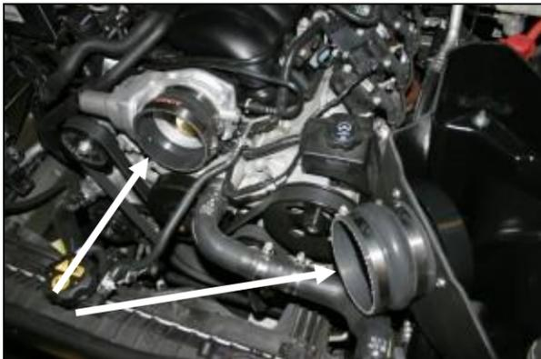
14. Install the hump hose onto the filter adapter using two #72 hose clamps. Next install the reducing coupler with one #60 hose clamp on the throttlebody and one #72 hose clamp on the large end.
