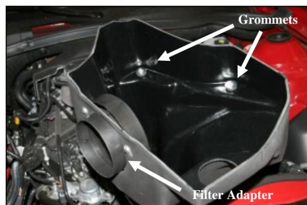
**8.** Reinstall the two steel sleeves and grommets into the Airaid Cold Air Box (CAB) (#4). Next install the filter adapter (#5) into the CAB as shown using three 1/4-20 button head bolts (#9), and 1/4" flat washers (#11). Refer to the line drawing above for details.
