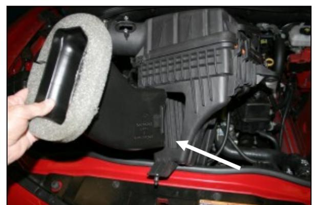
**6.** Squeeze the sides of the factory intake scoop and remove it from the factory airbox. It will be reused in step #10.
