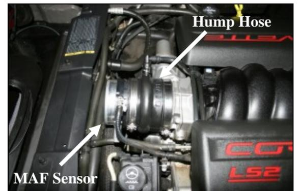
9. Install the hump hose with the #64 hose clamp on the throttlebody. Adjust it so that the breather hose aligns with the barbed fitting, and reconnect the breather. Tighten the hose clamp on the throttlebody. Reinstall the MAF sensor into the hump hose making sure the "Flow" arrow is pointing towards the engine. Tighten the remaining hose clamp.
