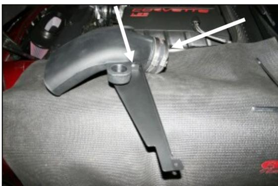
7. Attach the two air dams (#s 5&6) to the Airaid intake tube as shown using two 8-32 x 3/8" screws (#8), and two #8 flat washers (#10). Leave the screws slightly loose for adjustment later. Refer to the line drawing at the top of this page for reference. Next install the supplied coupler (#4) onto the Airaid intake tube as shown using two #60 hose clamps (#13). Tighten only the clamp on the tube.
