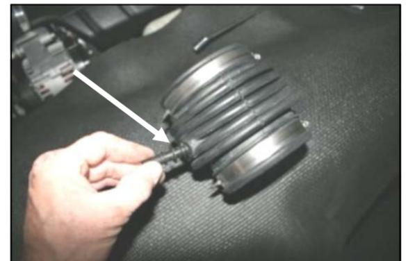
3. Remove the barbed fitting from the factory coupler. It will be reused in step #4.
