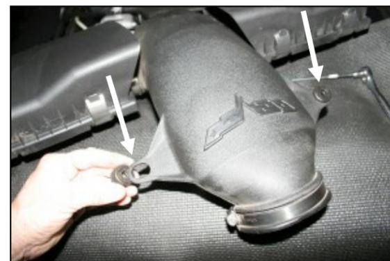
5. Remove the two factory grommets from the factory intake tube. They will be reused in step #6.
