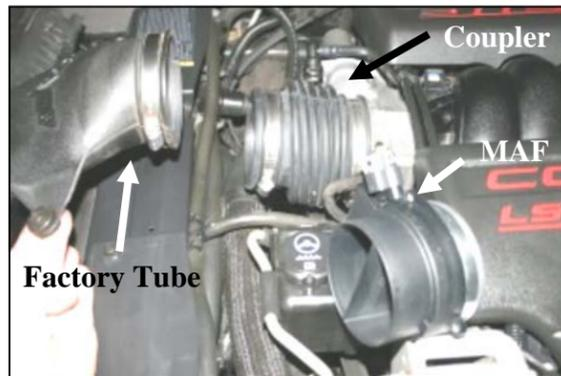
2. Lift the factory intake tube up and remove the Mass Air Flow (MAF) sensor from the coupler and slide it out of the way. Next remove the coupler from the throttlebody, and then remove the factory intake tube and filters from the vehicle as an assembly.
