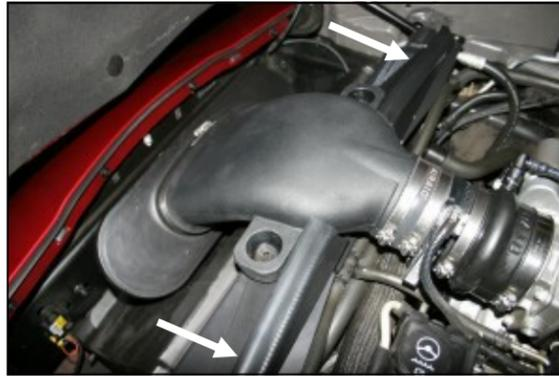
**11.** Install the supplied weather strips (#7) on top of the air dams as shown. Pull the Airaid Premium Filter up and secure it onto the Airaid intake tube with the supplied hose clamp.
