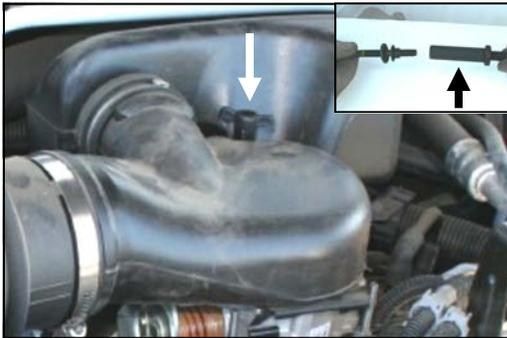
7. Using 6mm and 8mm wrenches, separate the factory rear throttle body stud as shown (reuse the top). Install the top of the stud onto the rear throttle body stud. Re-install the intake hat hold down nut. Tighten all bolts securely.
