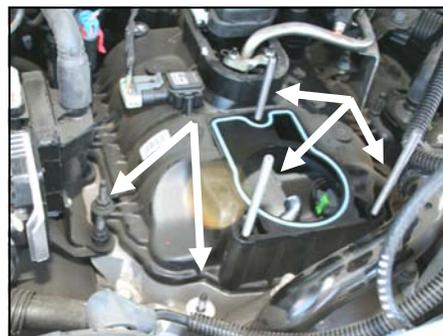
**3. With a 10mm deep well socket, remove the throttle body, throttle cable support bracket, and throttle cable bracket nuts. Using a 6mm 12 point socket, remove the rear stud from the throttle body. Disconnect the harness plugs on the throttle body.**
