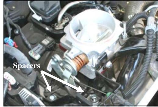
6. Install one 1/2" round spacer (#5) under each hole in the throttle cable bracket. Install the 6mmx 30mm bolt (#4) in the front hole, and the 6mmx 35mm bolt (#5) in the rear hole. Re-install the throttle cable bracket and nut onto the front of the throttle body. Install one 6 mm washer (#6) and 6mm nut (#7) onto each of the three throttle body studs. Tighten all bolts and nuts securely. Reconnect the harness plugs on the throttle body.
