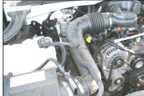
8. Re-install the intake tube, and tighten the hose clamps. Re-connect the breather hose elbow to the intake hat. **Re-connect the negative battery cable!**
