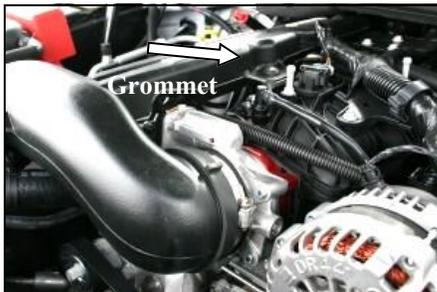
9. Re-install the intake tube using caution to center the intake tube hole over the previously installed grommet. Some adjustment may be required to seat the grommet correctly back into the intake tube. Tighten the hose clamps on the tube. Re-connect the breather tube. Re-install the plastic holder from step #1. Re-install the beauty cover.
