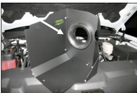
**8.** Assemble the Cool Air Dam panels (CAD) (#2 & #3) using five 6-32 x 5/16" screws (#10), #6 flat washers (#11), and 6-32 keps nuts (#12). Next install the air filter adapter (#5) into the panels as shown with the hole for the Mass Air Flow sensor facing up, using three 1/4 - 20 x 1/2" button head bolts (#14), and 1/4" flat washers (#15). Apply the Airaid Foil Decal onto the Panel as shown.
