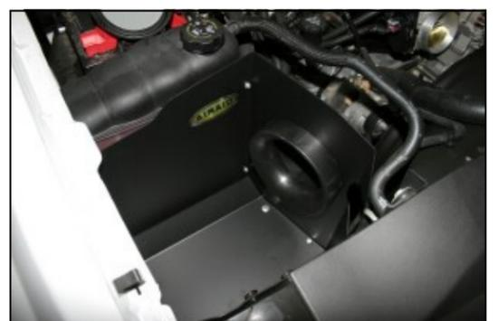
**9.** Install the Airaid CAD assembly into the vehicle replacing the factory airbox. Secure the CAD using four M6 x 1.25 Hex Bolt (#16), and 1/4" flat washers (#15). Do not over tighten the four bolts.
